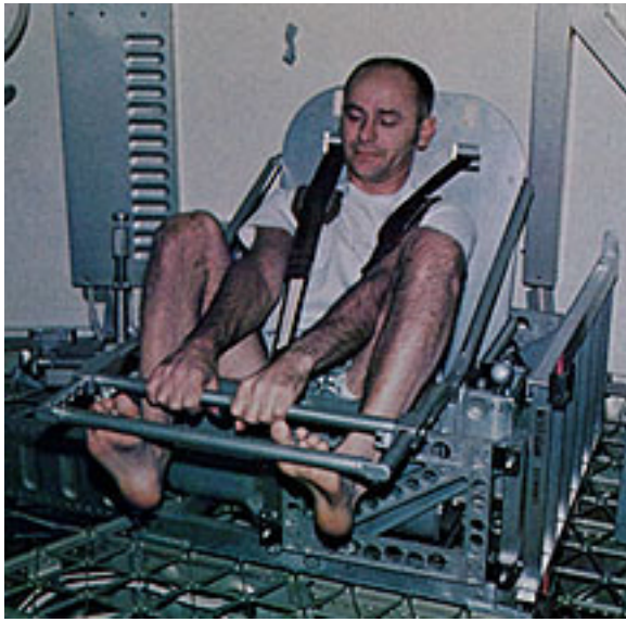
Figure 3. Spring-loaded Chair Device for Measuring Astronaut's Mass
