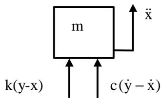
Figure 2. Free-body Diagram
