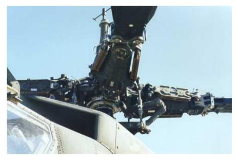
Figure 4. Main Rotor Hub
