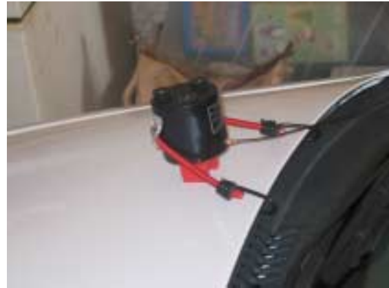
Figure 6. Shaker Mounted on Taurus Hood
