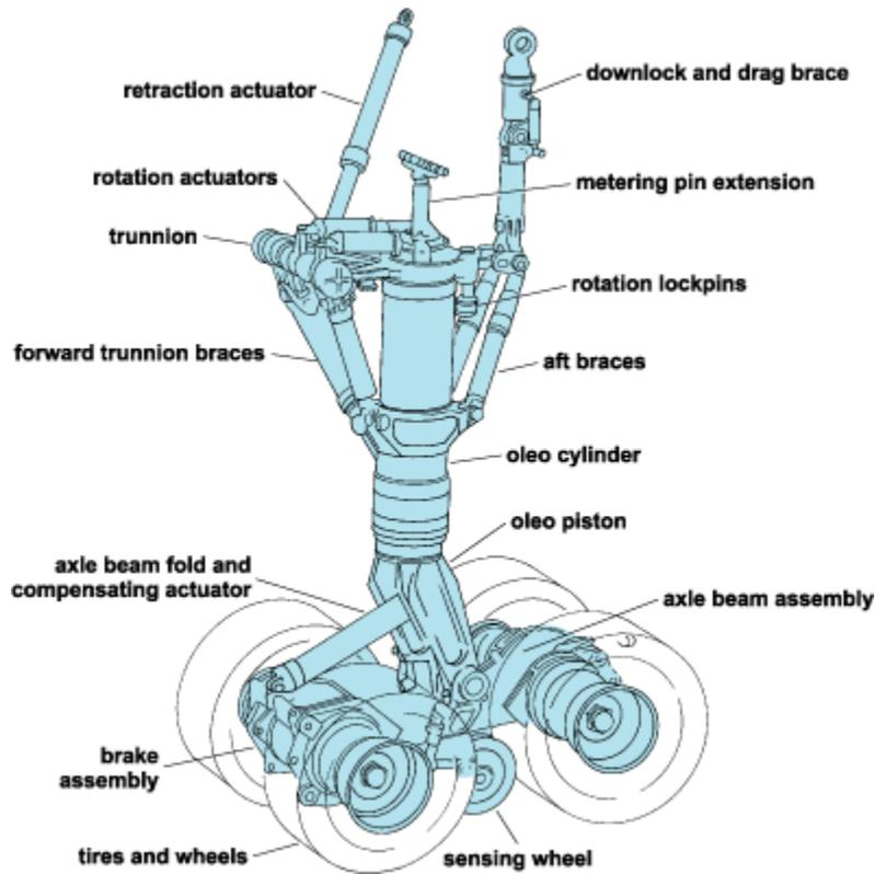
Figure 1. Main-wheel Bogie for the XB-70A aircraft
