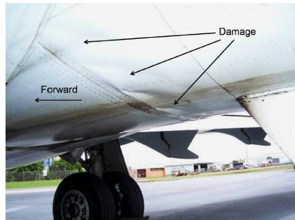
Figure 2. Fuselage Skin Panel Damage
