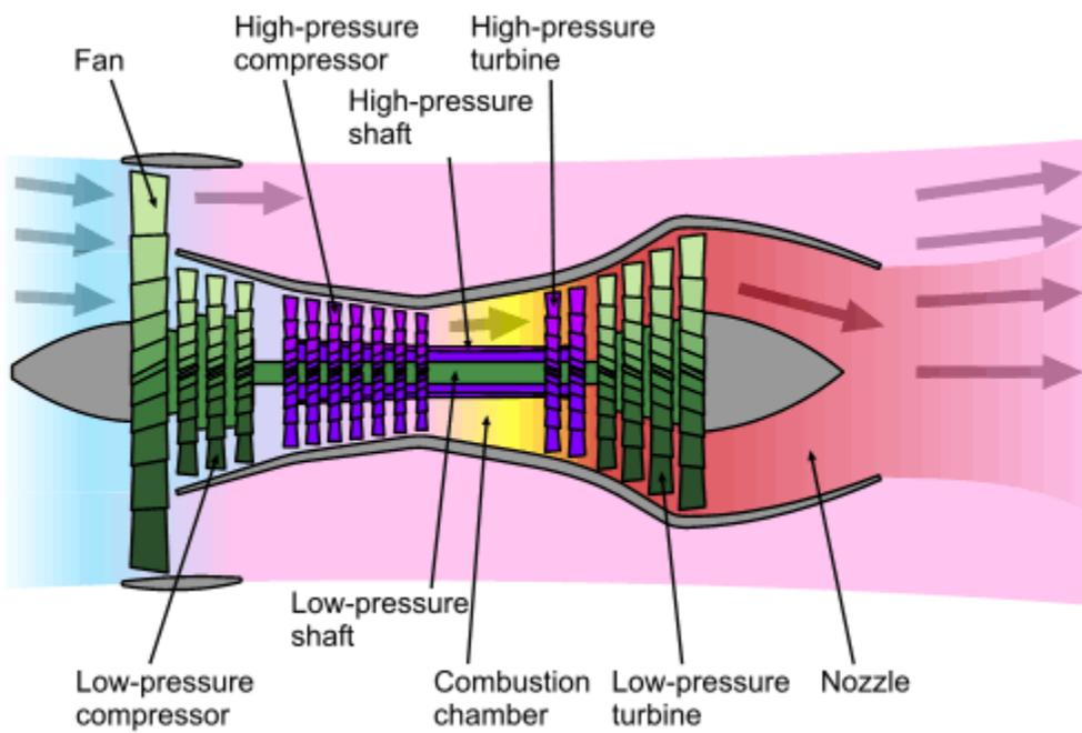
Figure 4. Turbofan Engine Subsystems
