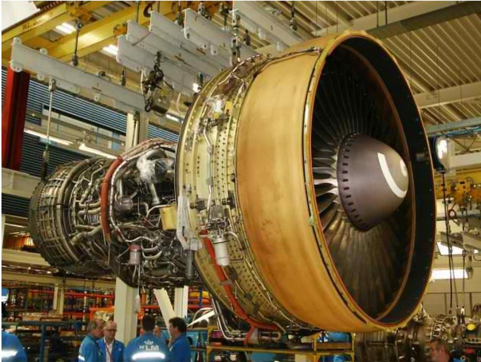
Figure 1. General Electric CF6 Turbofan Engine
