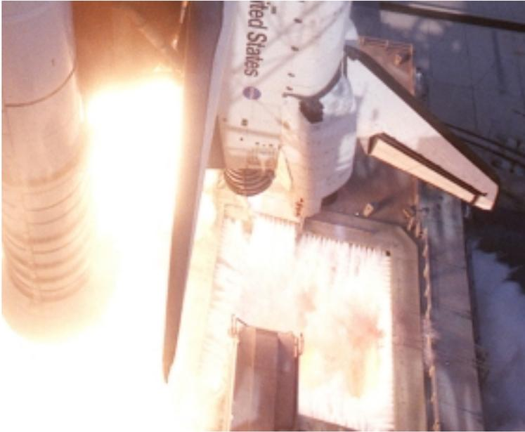
Figure 2. Main Engine Exhaust Hole and Water Spray
