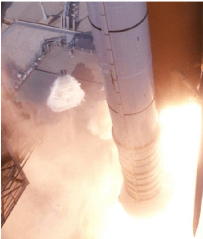
Figure 3. Rainbird, Left of the Solid Rocket Booster
