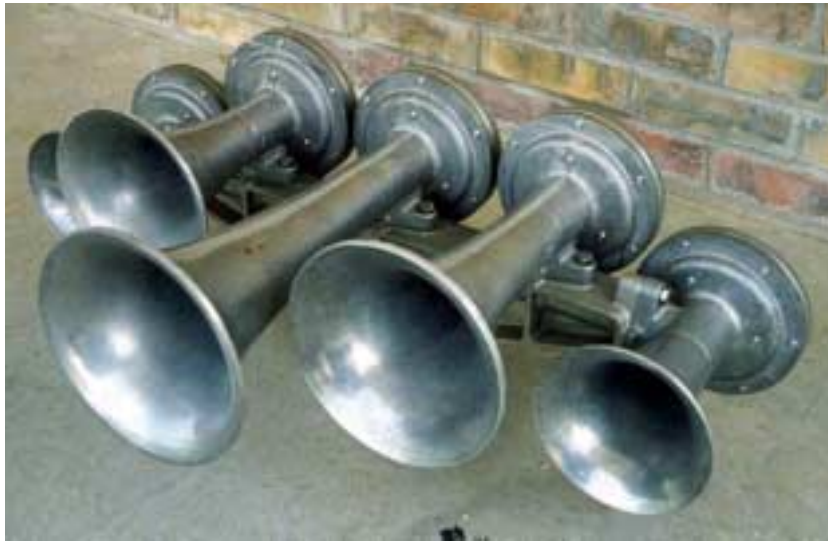
Figure 2. K5LA Horn with Five Chimes (Photo courtesy of Brent Lee)
