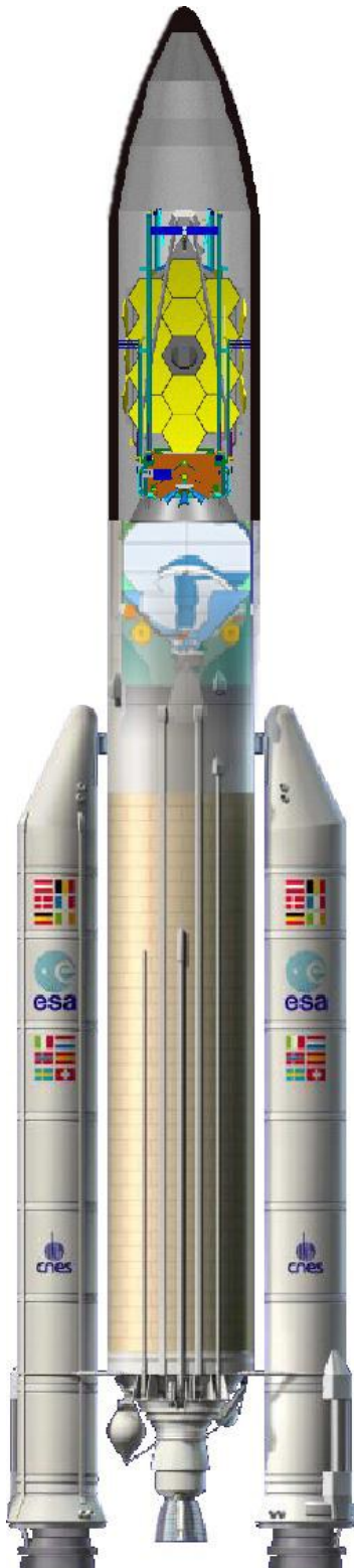
Figure 2. Ariane 5 with Stowed JWST
