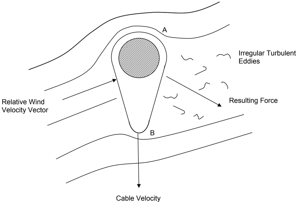
Figure 2. Wind Blowing against an Ice-Coated Cable
