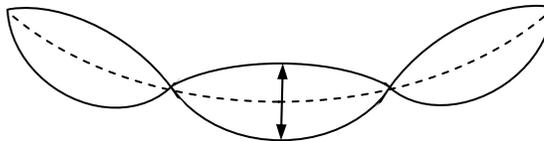
Figure 3. Possible Galloping Modes for a Subspan, Exaggerated
