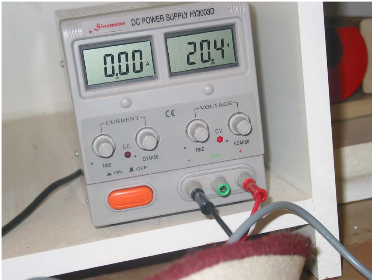
Figure 7. DC Power Supply for Displacement Sensor
