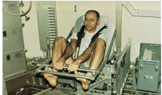
Astronaut Alan Bean "weighs" himself on the body mass measuring device, aboard Skylab.
