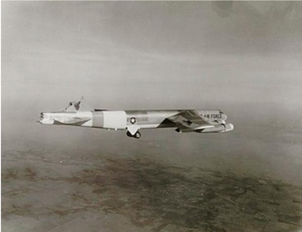
Figure 4. B-52 with Missing Vertical Stabilizer
