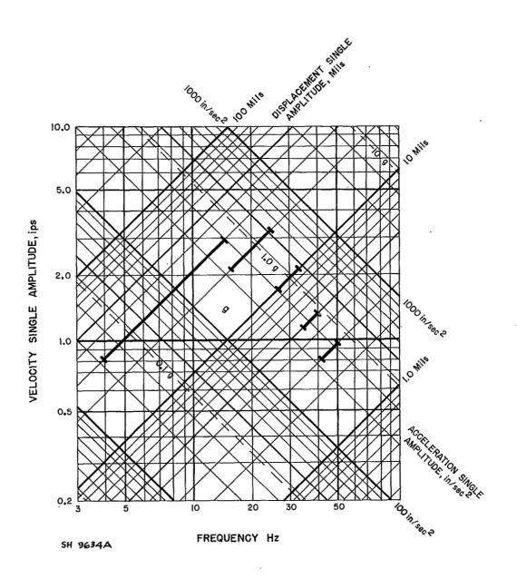
Figure 1 - Type I environmental vibration limits (graphical presentation expressed in displacement, velocity and acceleration).
