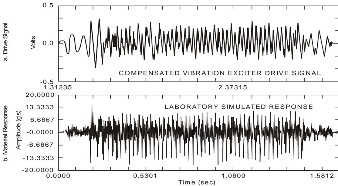
FIGURE 519.5A-6. Compensated vibration exciter drive signal along with resulting test item response.
