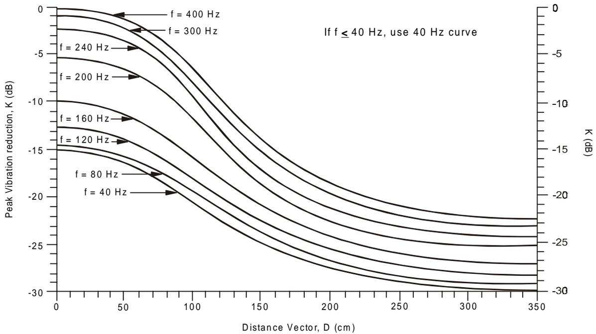
FIGURE 519.5D-8. Gunfire peak vibration reduction with distance.
