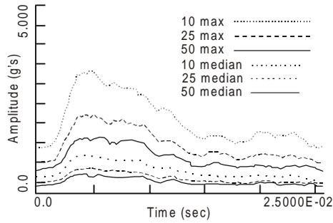
**FIGURE 519.5B-13. Smoothed simulation root variance estimates for the time-varying standard deviation for simulated ensemble sample sizes of 10, 25, and 50 sample time histories maximum and median  $N_p = 10, 25,$  and 50.**
