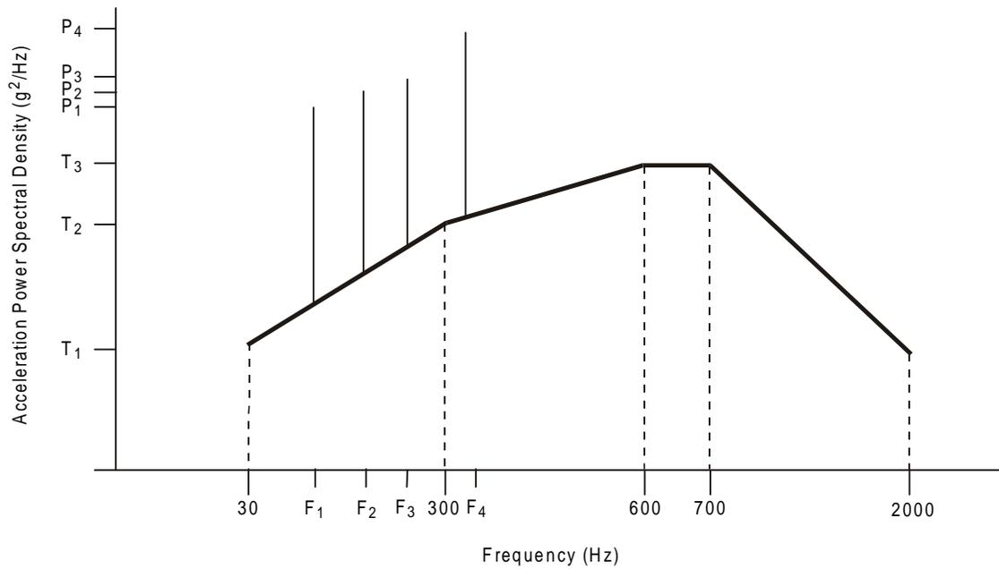
**FIGURE 519.5D-1. Generalized gunfire induced vibration spectrum shape.**
