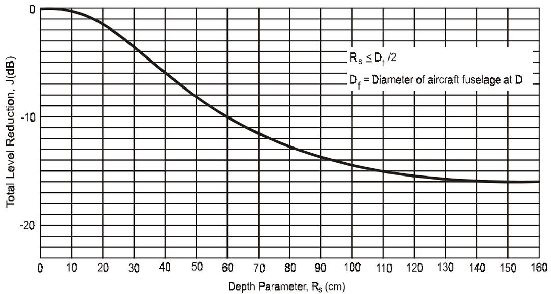
**FIGURE 519.5D-6. Test level reduction due to depth parameter.**
