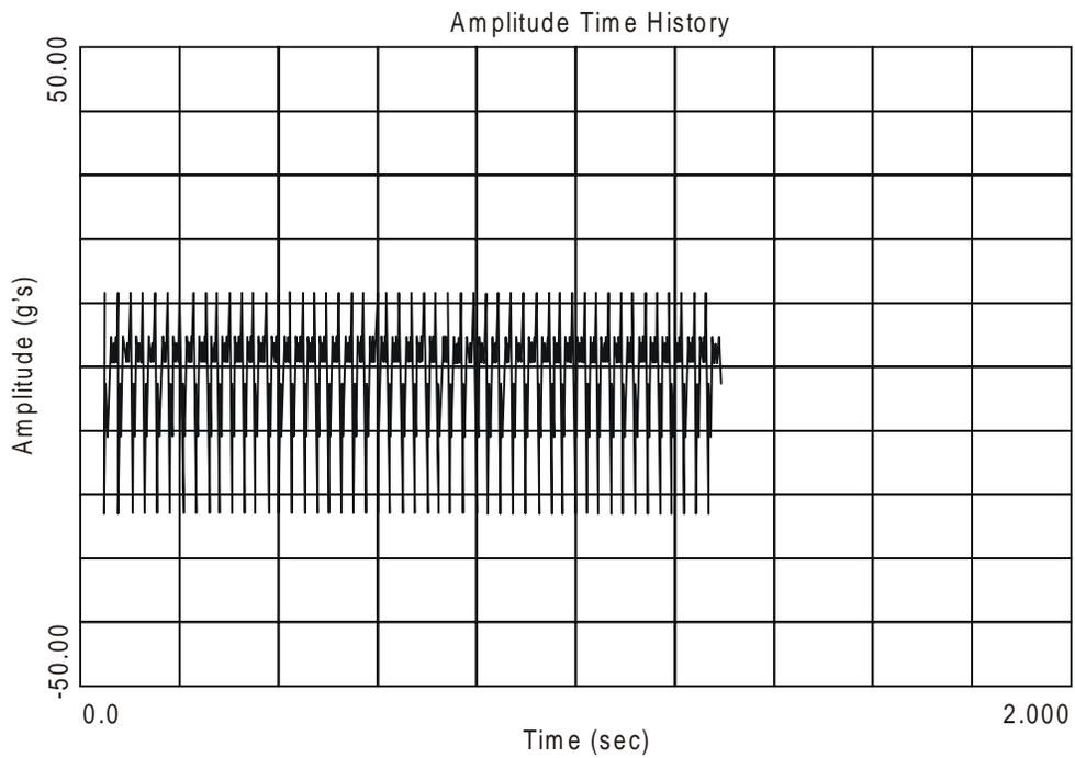
**FIGURE 519.5C-4. SRS pulse gunfire simulation-analytical pulse concatenation.**
