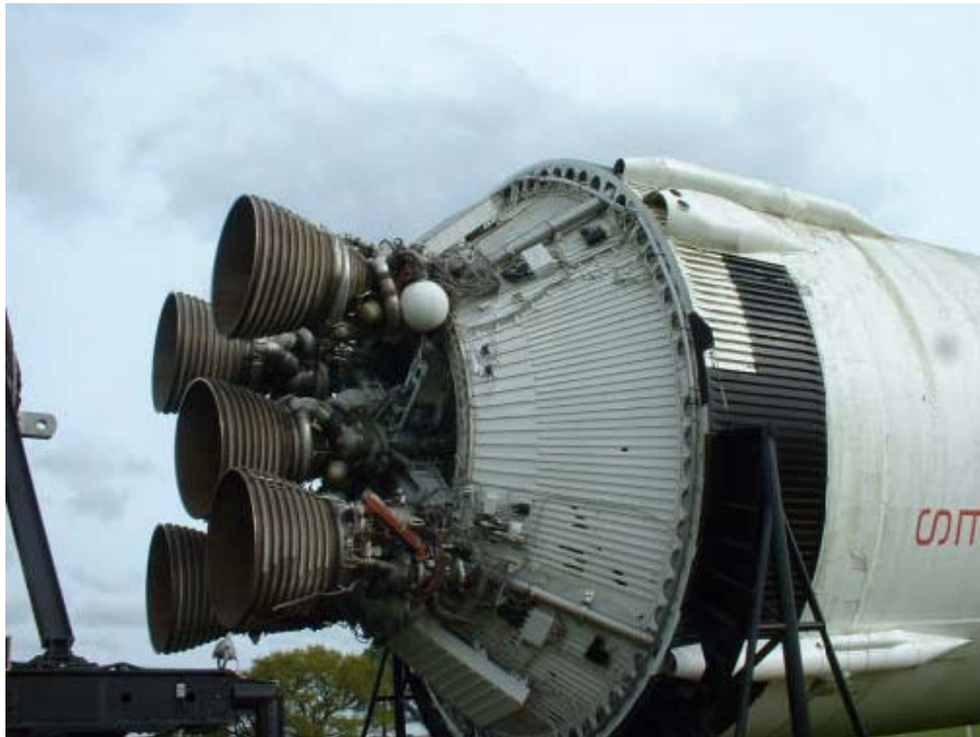
Figure 8. Saturn V Second Stage S-II Close up, J-2 Engine Cluster 15
