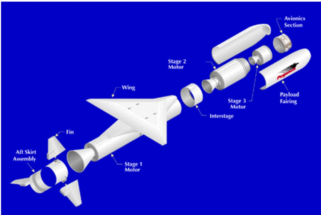
Figure A-1. Diagram of the Pegasus Launch Vehicle
