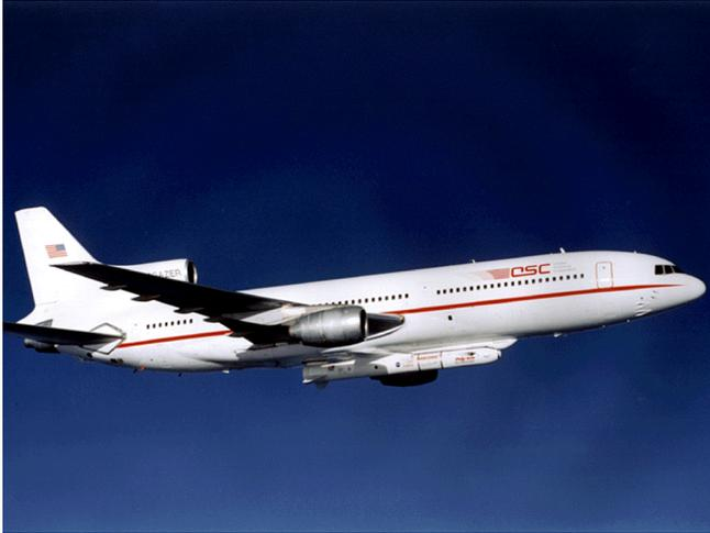
Figure 1. Pegasus Carried underneath the L-1011 Aircraft
