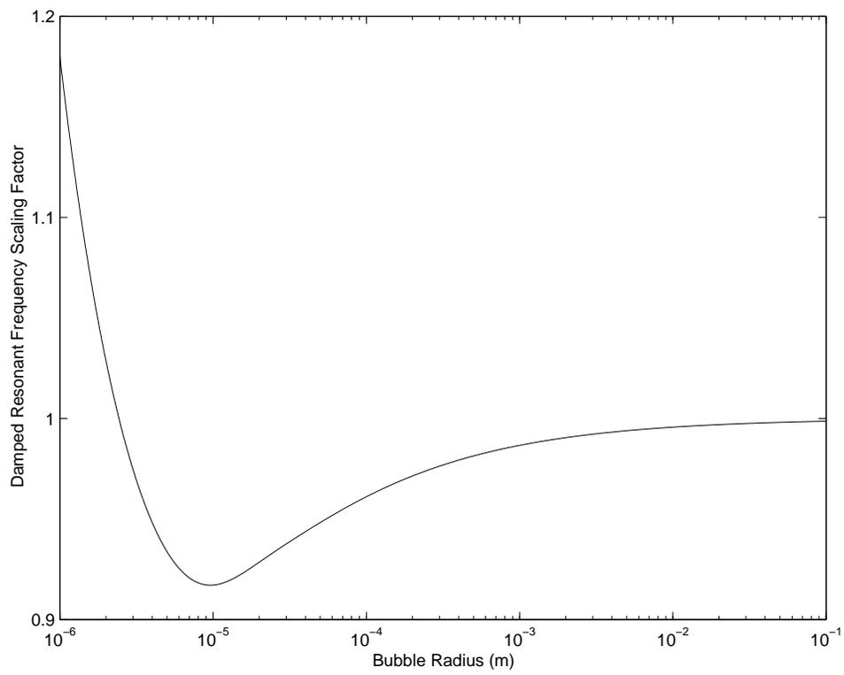
Figure 3: Damped resonant frequency scaling factor
