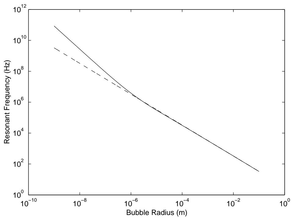
Figure 4: Resonant bubble frequency  $\omega_{0,d}/2\pi$
