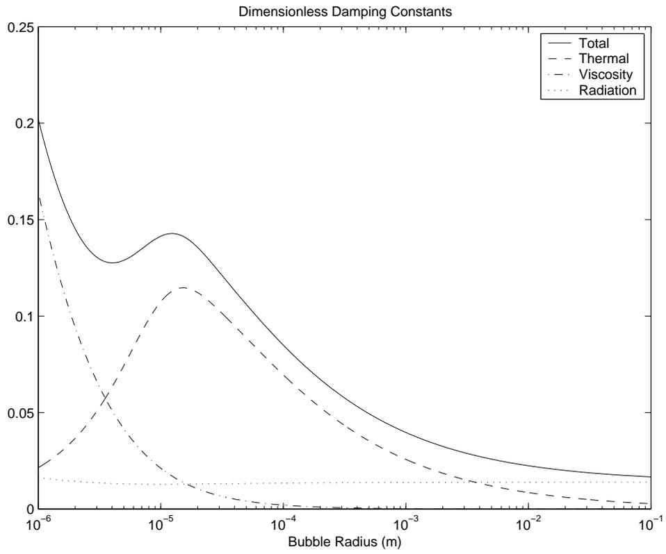
Figure 2: Resonant bubble damping coefficient
