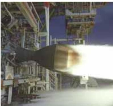
Figure 1. Fastrac Engine, Static Fire Test
