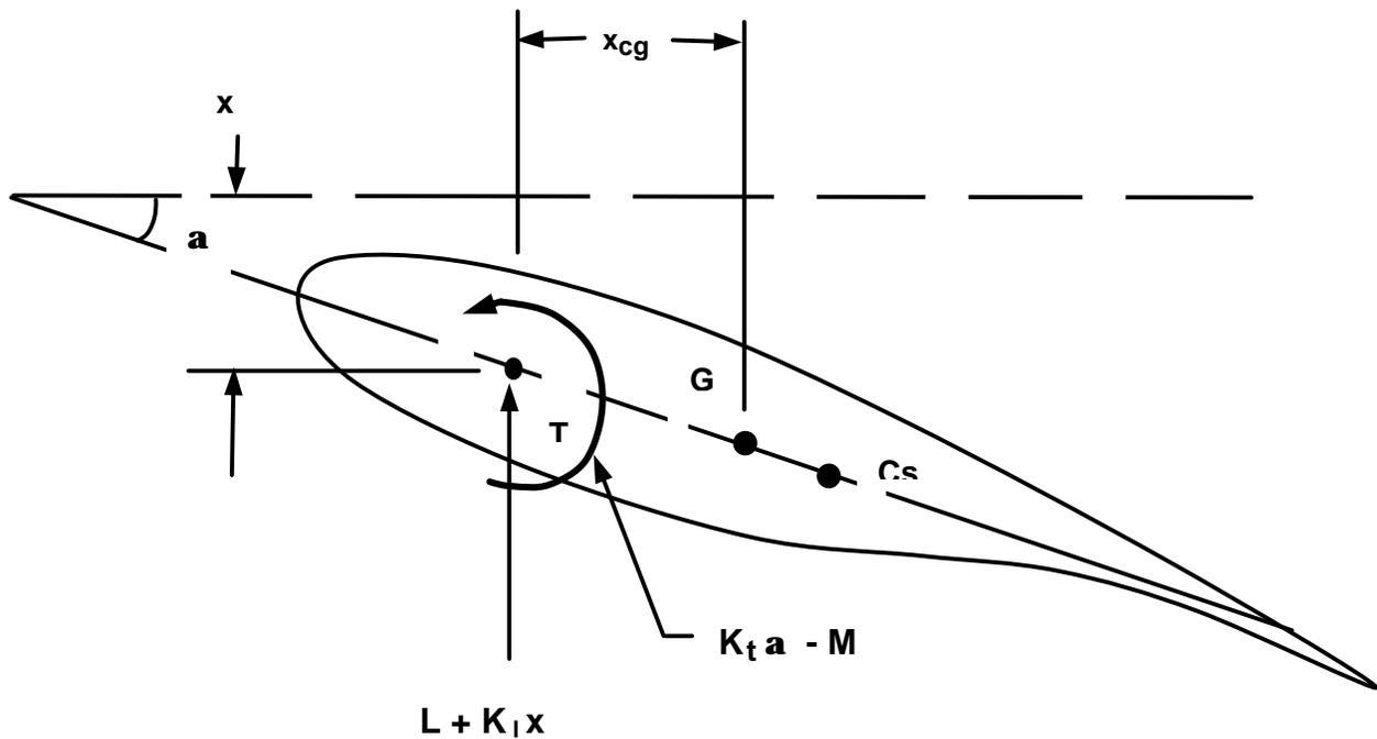
L is the aerodynamic lift force acting through the center of twist.
