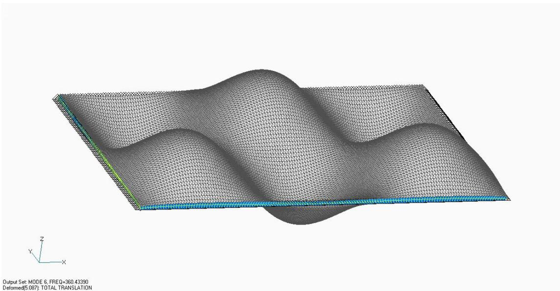
Figure D-4. Typical FEA Mode Shape,  $f_n = 362$  Hz
