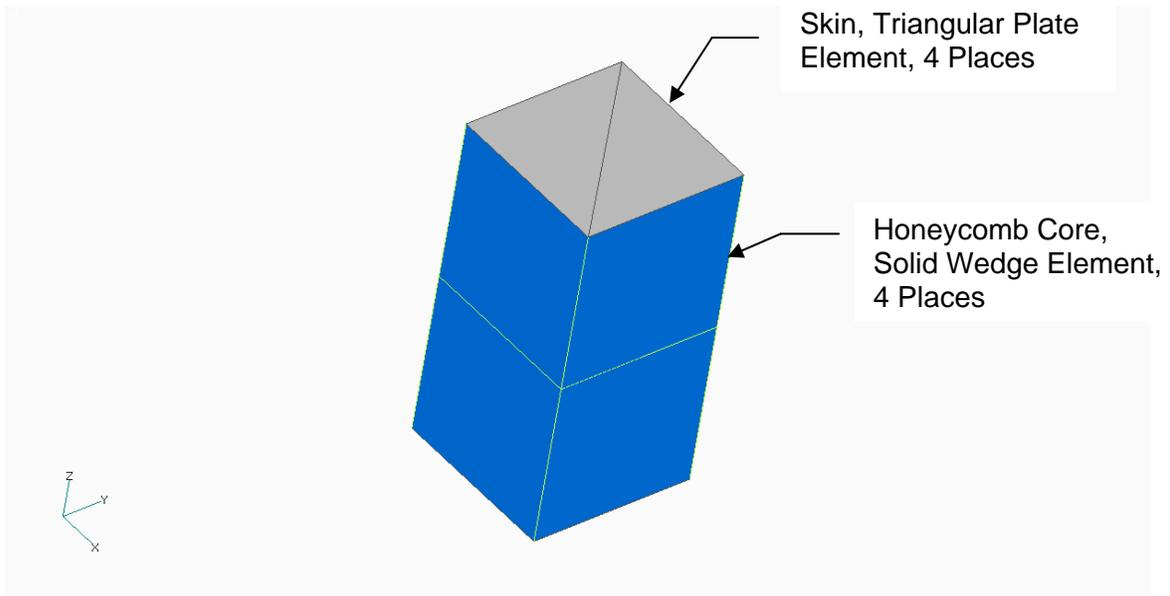
Figure D-2. Manually Constructed Laminate for FEA
