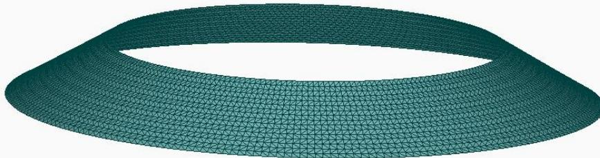
Figure C-2. Mode 1,  $f_n = 39.6$  Hz
