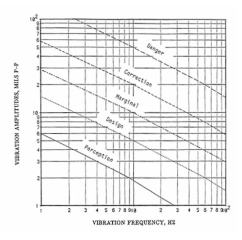
Figure 1. Allowable Piping Vibration Levels versus Frequency
