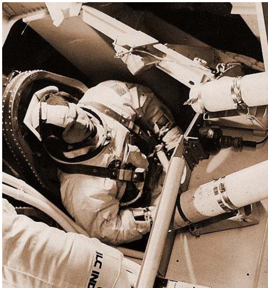
Astronaut Frank Borman, commander of Apollo 8, rides the centrifuge at Manned Space Center, Houston, Texas. Special instrumentation was added to simulate pogo effects that might be encountered during actual flight. Photo courtesy of NASA.
