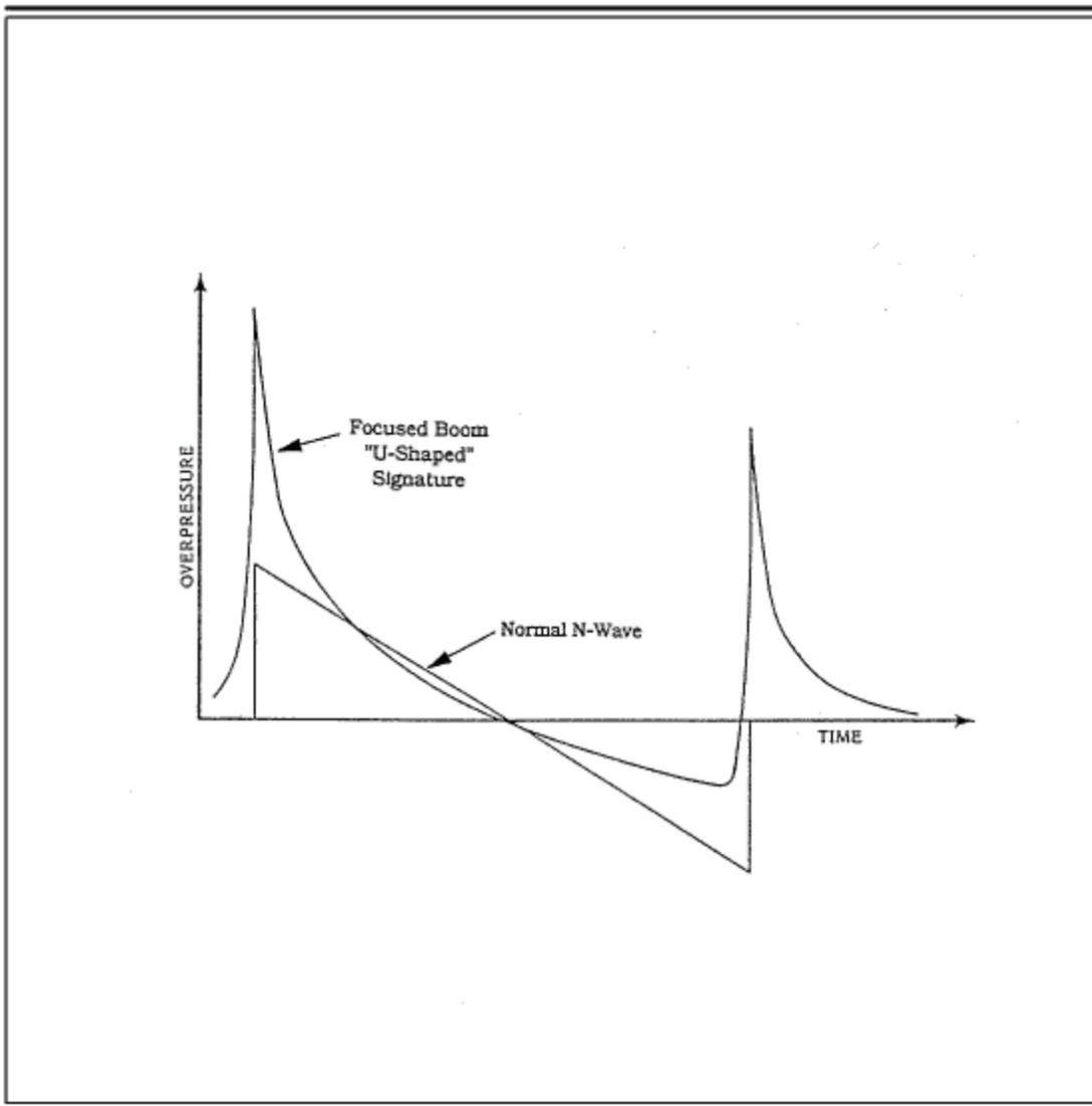
**Focused U-Wave and Unfocused N-Wave Boom Signatures**
