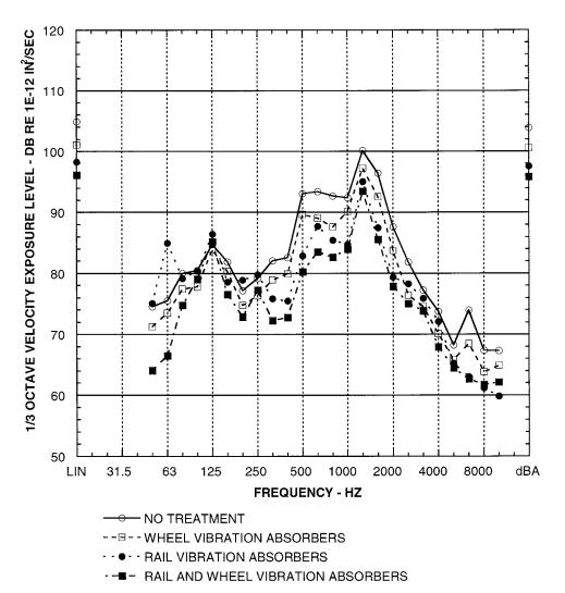
Figure 11. Rail head transverse vibration.
