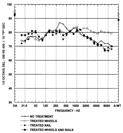
Figure 19. One-third octave SELs for eastbound 25-mph test vehicle at East Portal test section.
