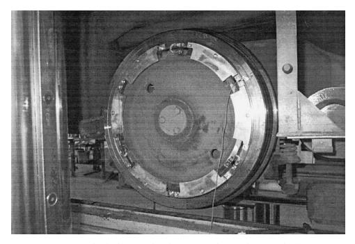
Figure 2. Tri-Met wheel vibration absorbers mounted on Bochum 54 wheels.
