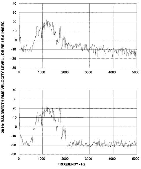
Figure 12. Auto-spectra of rail vertical vibration at two adjacent tie spaces prior to train passage.
