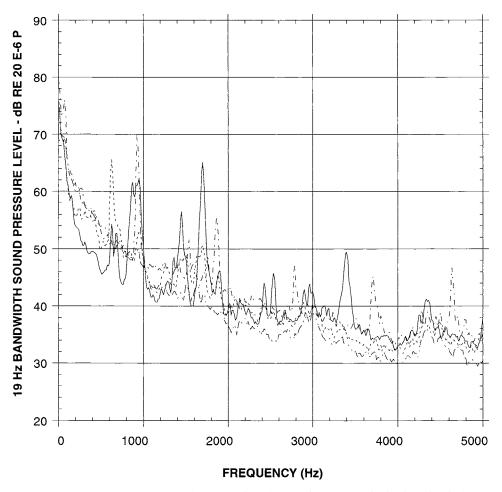
Figure 17. Fourier spectra for four samples of wayside noise at the high rail side for Car No. 9 with untreated Bochum 84 wheels.
