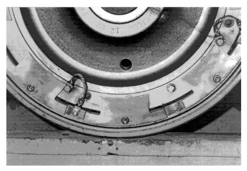
Figure 1. VSG vibration absorber attached to NJT Bochum 84 resilient wheel.
