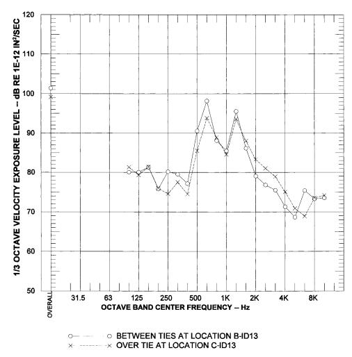
Figure 15. Vertical rail head vibration over tie and between ties for 45 mph vehicle with treated wheels on treated rail.
