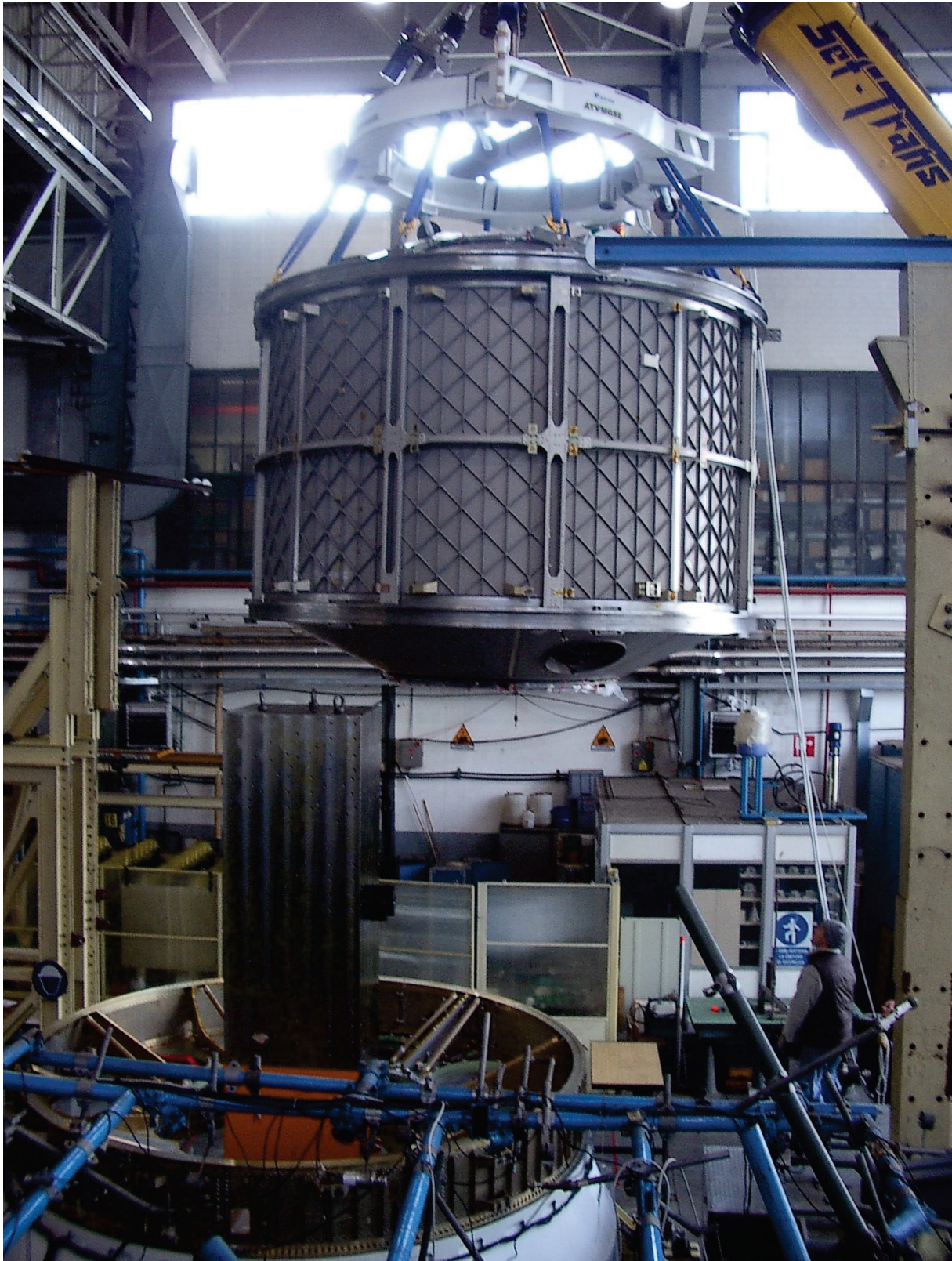
Figure 7-3: Setting of ATV primary structure static test
