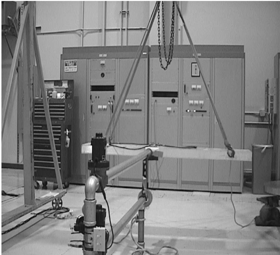
Figure 16. Shock Test Set-up
