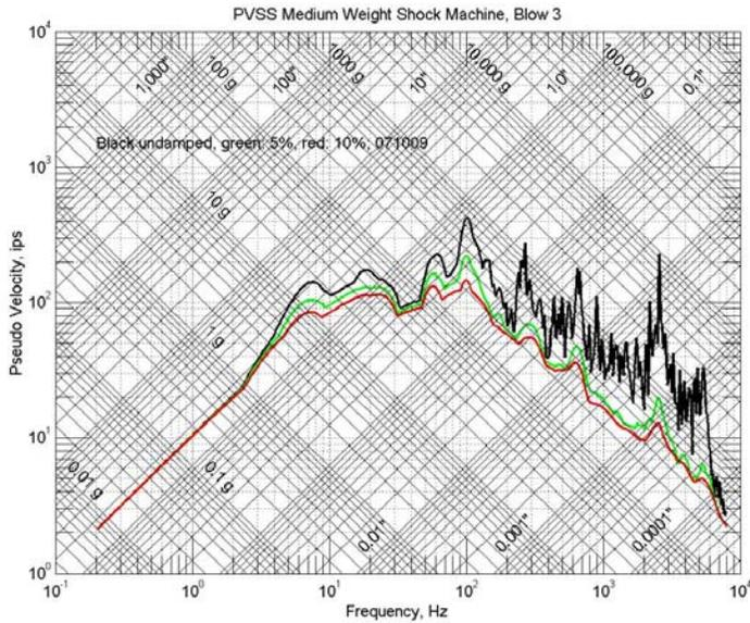
Figure 7b. The maximax PVSS of blow 3 on the Navy Medium Weight Shock Machine,.
