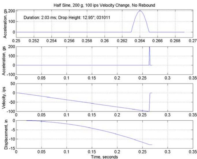
Figure 4a. Time history and integrals for a 100 ips, 200g, drop table half sine shock. The uppermost subplot is an expanded version of the second subplot, included to show detail of the half sine shock.
