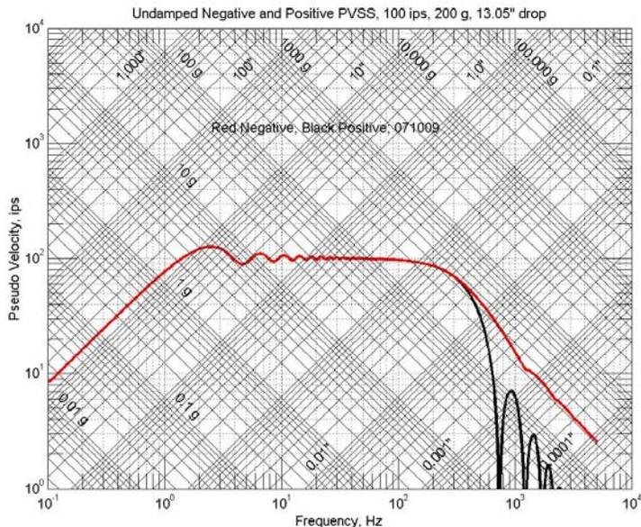
Figure 4c. Positive and negative PVSS for the undamped 100 ips, 200g, half sine shock of Figure 4a.
