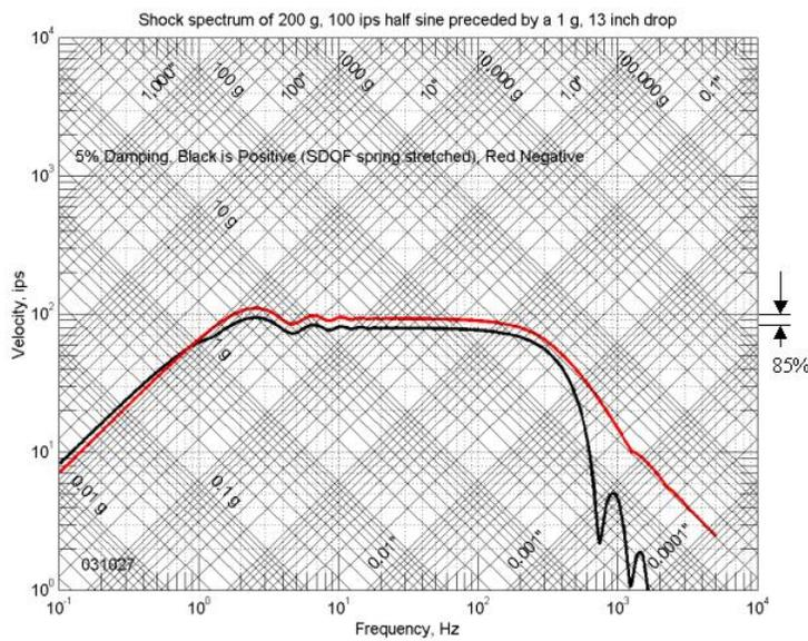
Figure 4d. Positive and negative PVSS for a 5% damped 100 ips, 200g, half sine. The negative spectrum exceeds the positive everywhere except at low frequencies during the drop.
