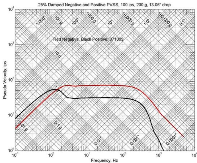
Figure 4e. Positive and negative PVSS for a 25% damped 100 ips, 200 g, half sine. The negative spectrum strongly exceeds (over twice) the positive in the high PV plateau.
