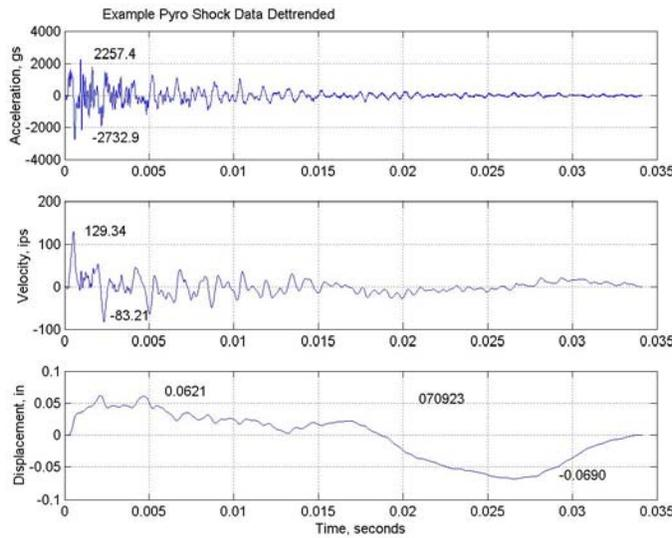
Figure 6a. This is a pyroshock detrended data segment with peak values printed on graph.
