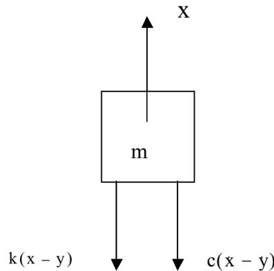
Figure 3, The free body diagram of the mass.
