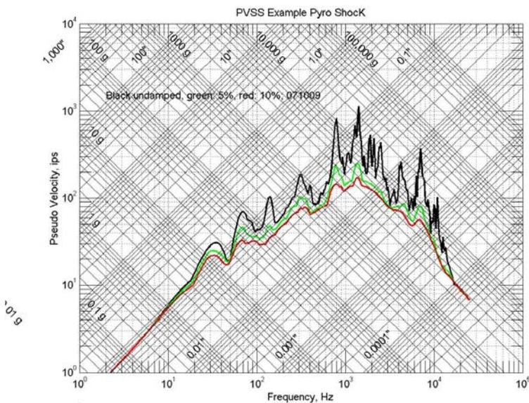
Figure 6b The example pyroshock PVSS with 0%, 5%, and 10% damping.
