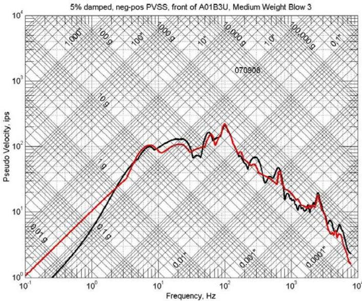
Figure 7d The 5% damped posneg PVSS of blow 3 on the Navy Medium Weight Shock Machine.
