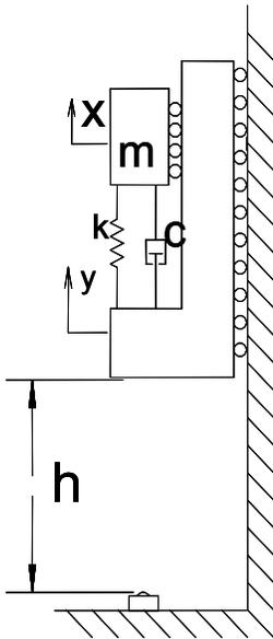
Figure 2, The shock table wheeled bogey with a single degree of freedom system
