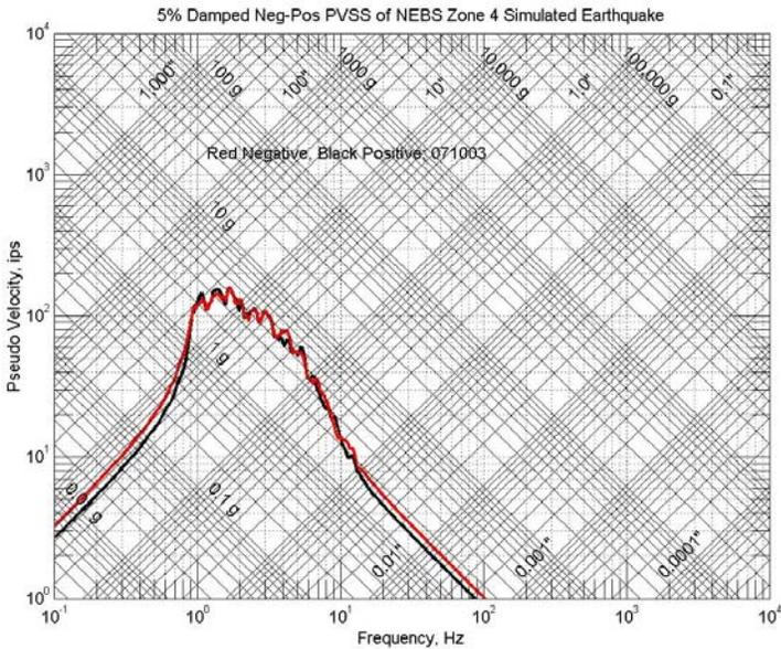
Figure 5d. The 5 % damped posneg PVSS of the NEBS Zone 4 acceleration of Figure 5a. Now 25% damping
