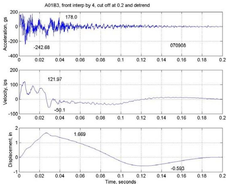
Figure 7a. The time history and integrals from Blow 3 of a Navy Medium Weight Shock Machine test.
