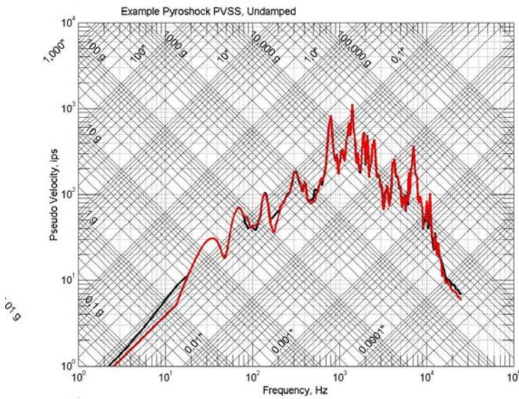
Figure 6c Pyroshock example undamped posneg PVSS.
