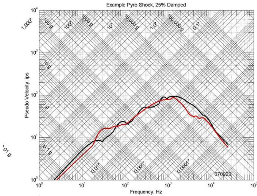
Figure 6e Pyroshock example 25% damped posneg PVSS. There are two regions with a significant lack of polarity.
