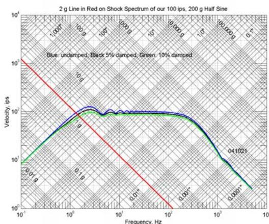
Figure 1. This is the PVSS on 4CP of a half sine shock with a velocity change on impact of 100 ips and a maximum acceleration of 200 g's. It occurs on a drop table shock machine with a 13 inch drop height and no rebound and with the table impacting a pad that causes a peak acceleration of 200 g's.
