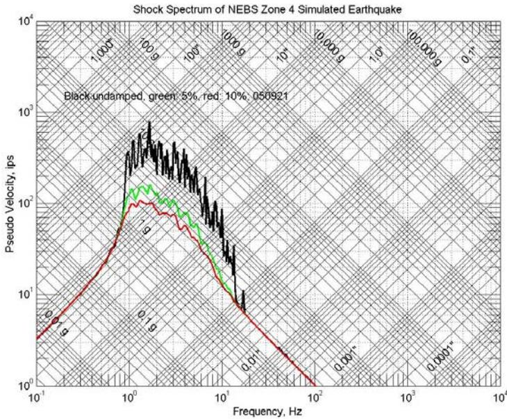
Figure 5b, The undamped, 5% and 10% damped PVSS of the NEBS Zone 4 Earthquake test time history [14].
