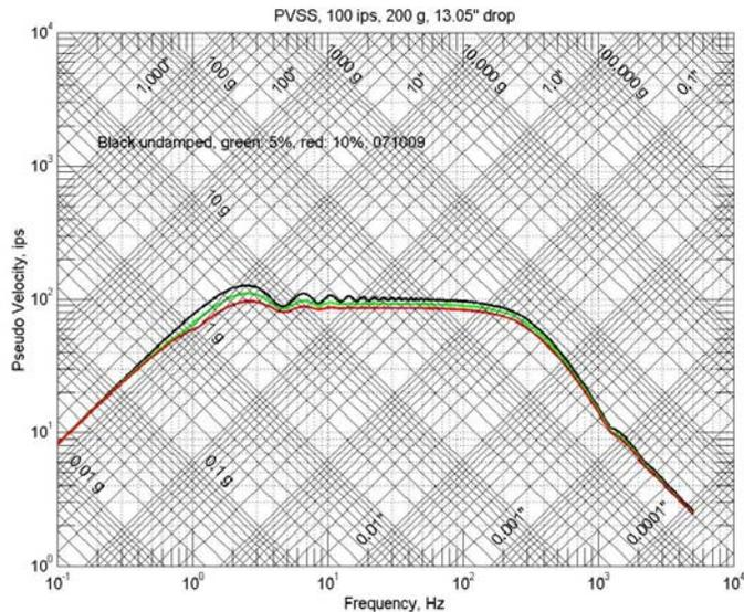
Figure 4b. Effect of Damping on the simple half sine shock. The undamped plateau, in black, is right on 100 ips. The 5% green plateau is at 93% or 93 ips. The 10% red plateau is at 86% or 86 ips. The low frequency asymptote is a constant displacement line at 13 inches, and the high frequency asymptote is on the 200 g constant acceleration line.
