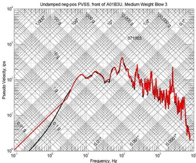
Figure 7c. The undamped posneg PVSS of blow 3 on the Navy Medium Weight Shock Machine.
