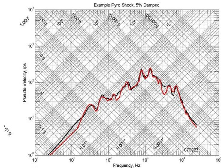
Figure 6d Pyroshock example 5% damped posneg PVSS.
