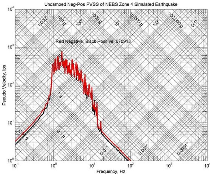
Figure 5c. The undamped posneg PVSS of the NEBS Zone 4 acceleration of Figure 5a.
