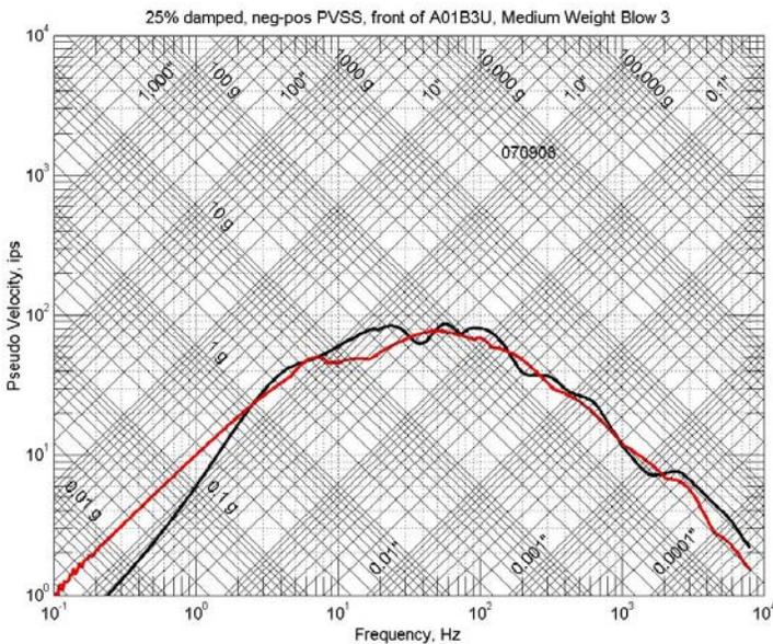
Figure 7e. The 25 % damped posneg PVSS of blow 3 on the Navy Medium Weight Shock Machine.
