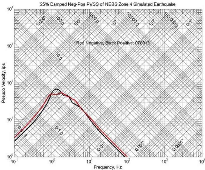
Figure 5e. The 25 % damped posneg PVSS of the NEBS Zone 4 acceleration of Figure 5a
