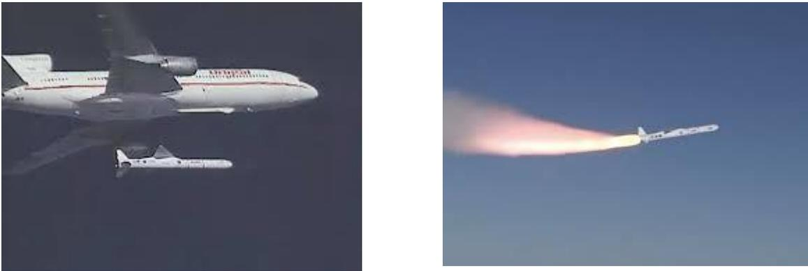
Figure 11.5. Pegasus Launch Vehicle, Drop & Stage 1 Burn
