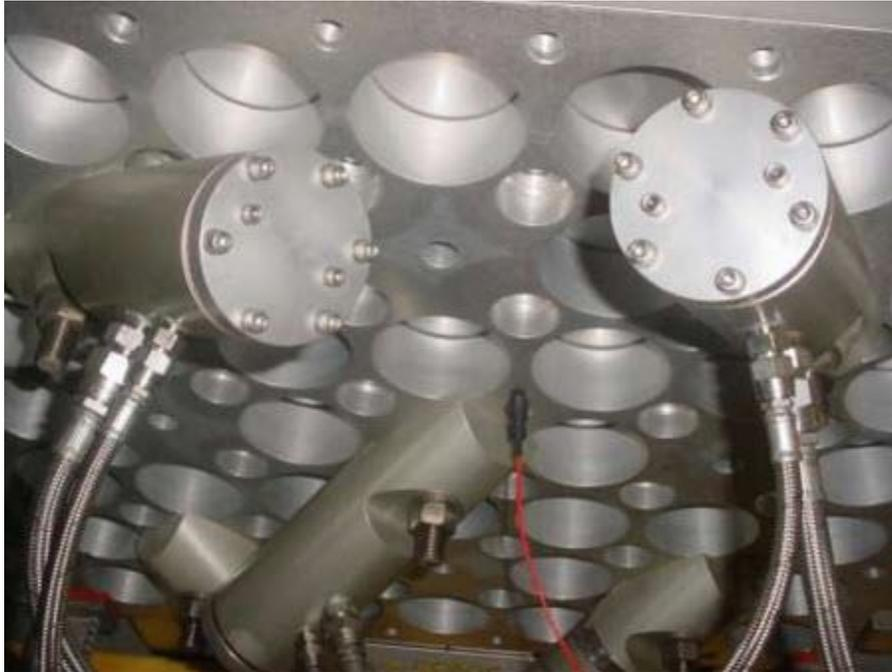
Figure 14.19. HALT/HASS Chamber Vibration Impactors
