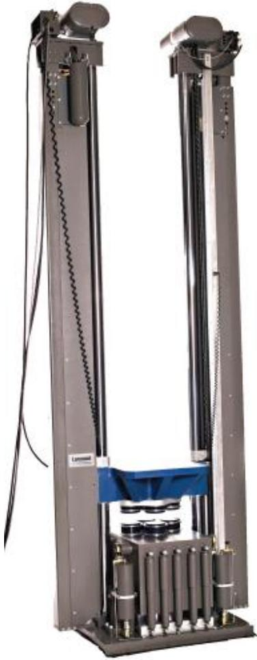
Figure 19.5. Drop Shock Test Machine, Initial Velocity Excitation
