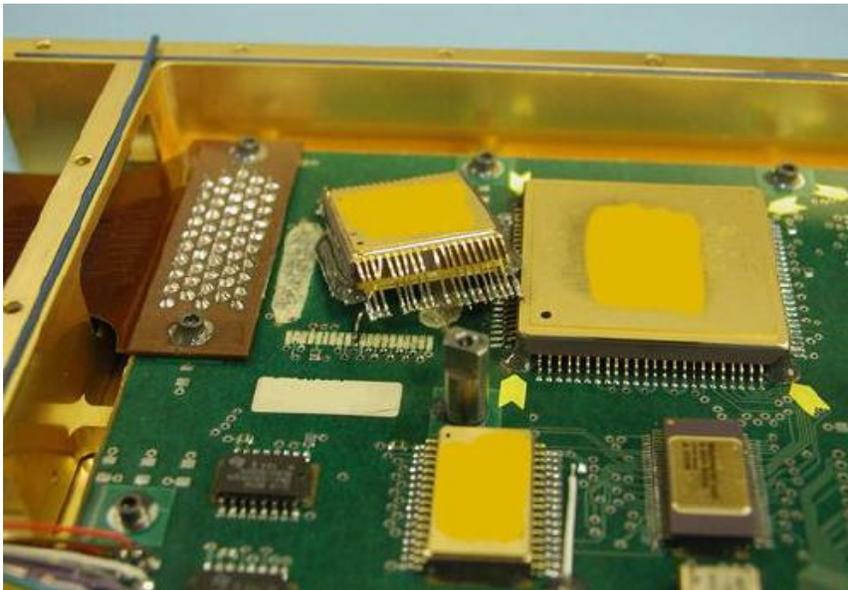
Figure 19.54. Shock Test Case History, Adhesive & Solder Joint Failure
