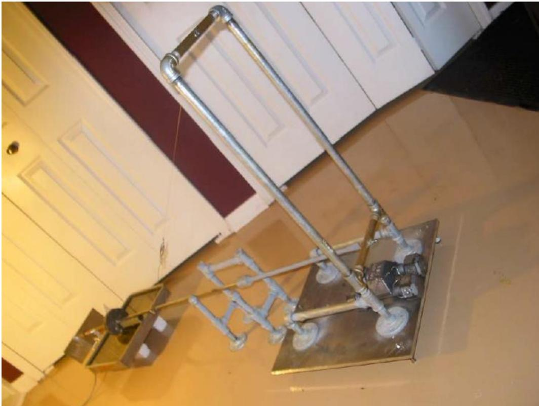
Figure 21.9. Author's Homemade Lehman Seismometer
