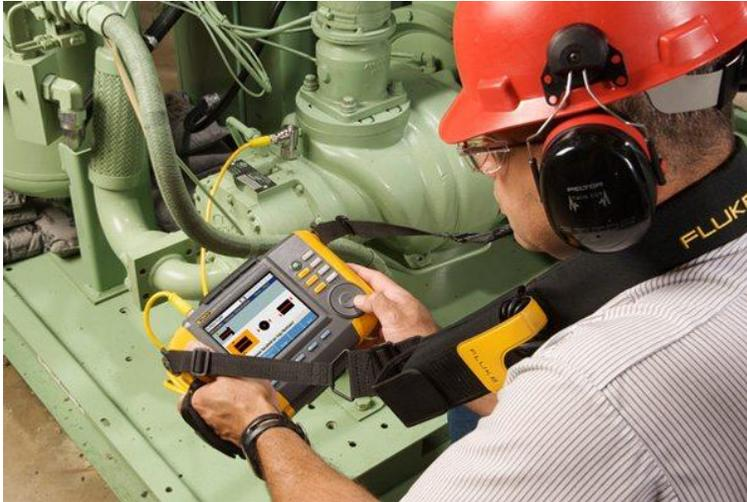
Figure 5.6. Vibration Monitoring for Predictive Maintenance
