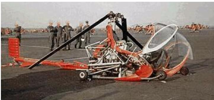
Figure 13.7. TH-55 Osage, Destroyed by Ground Resonance
