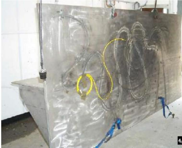
Figure 19.51. Near-Field Shock Simulation using a Plate
