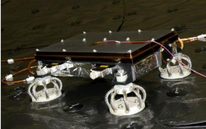
Figure 19.49. Sensor Electronics, Wire Rope Isolators (NASA/JPL photo)
