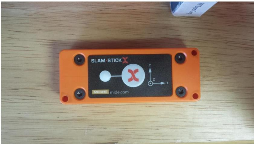
Figure 11.3. Slam Stick X, Triaxial Accelerometer & Data Logger, Shown on Book Shelf
