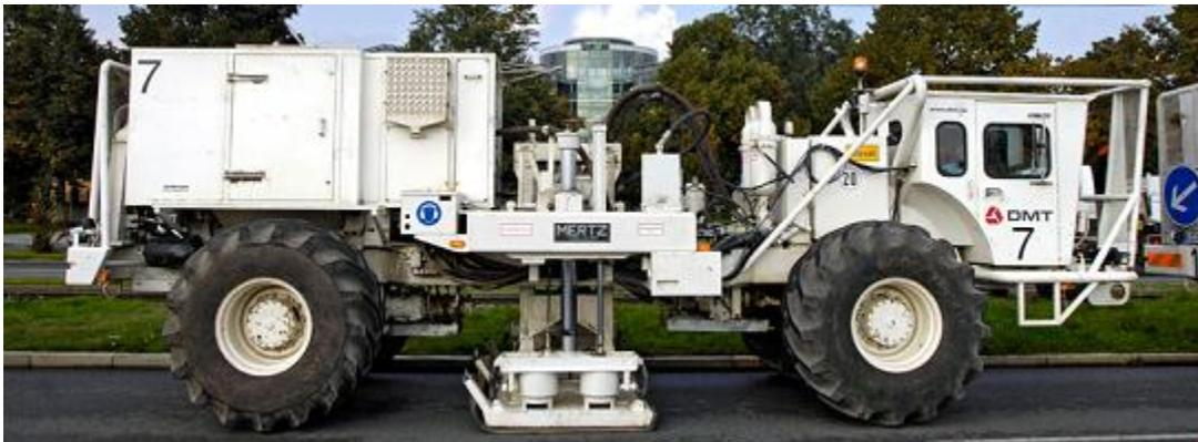
Figure 5.13. Thumper Truck, Applied Force
