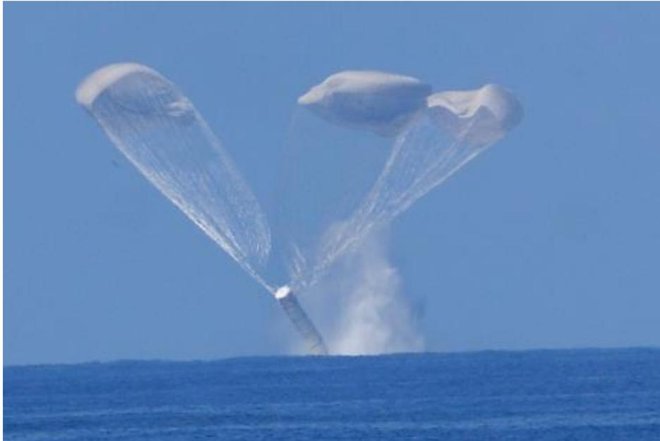
Figure 19.38. Solid Rocket Booster Water Impact Shock
