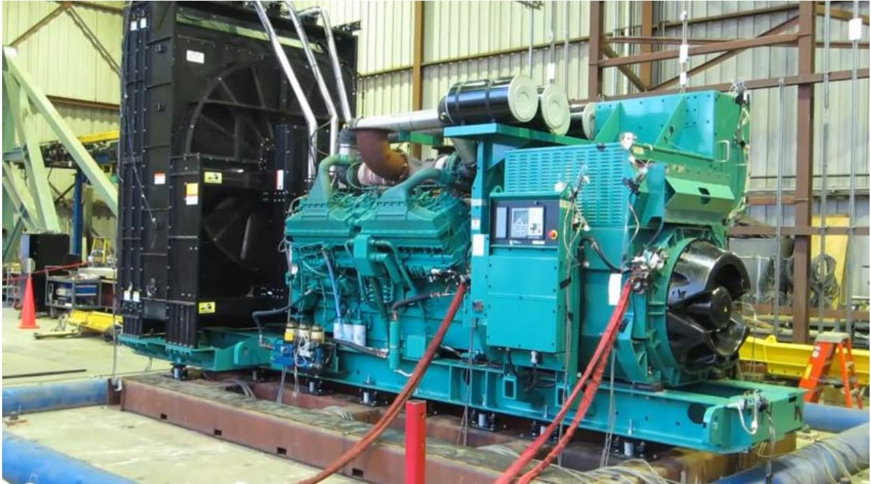
Figure 19.29. Electrical Power Generator Seismic Shock Test
