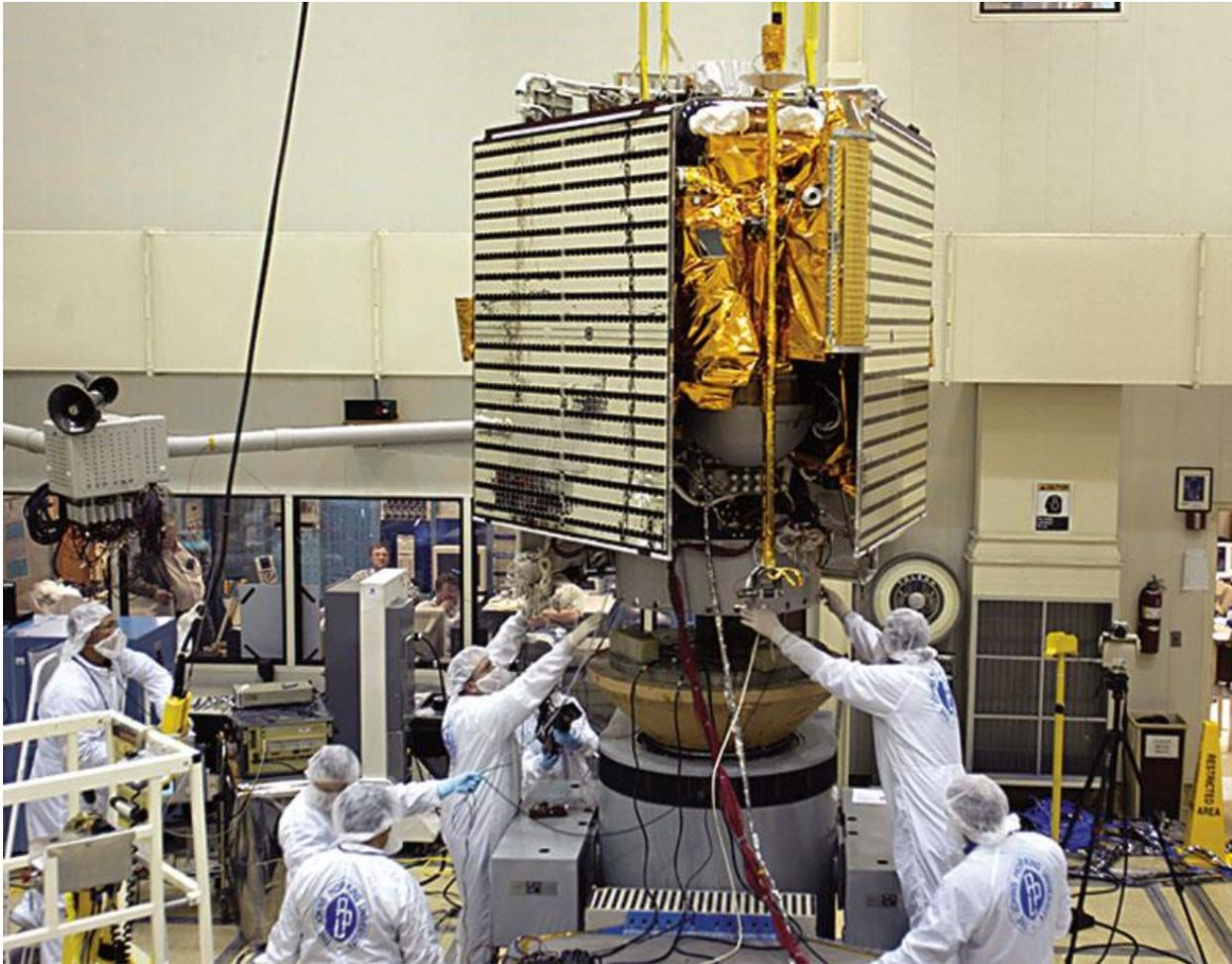
Figure 22.1. Shaker Table Vibration Test
