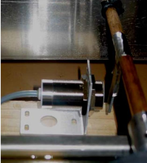
Figure 21.10. Non-contact Relative Displacement Sensor
