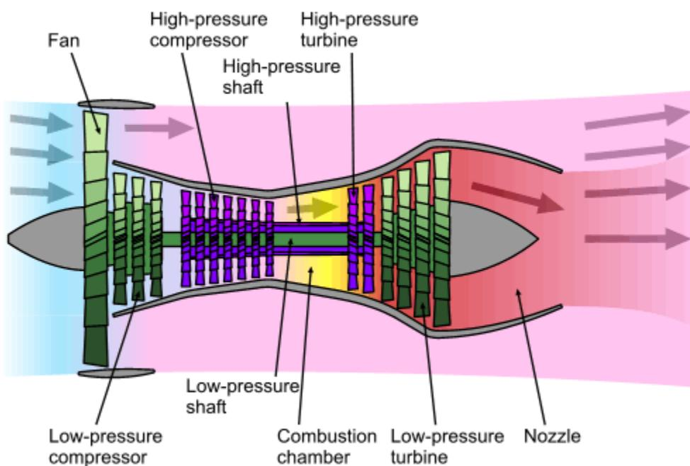
Figure A-3. Turbofan Engine Subsystems
