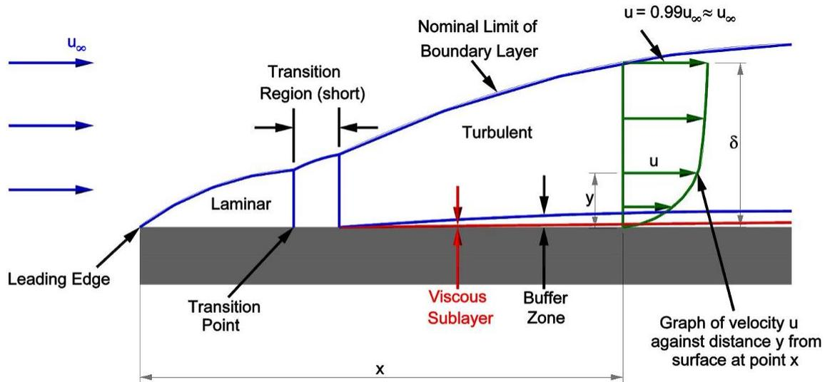
Figure 1. Boundary Layer on a Flat Plate
