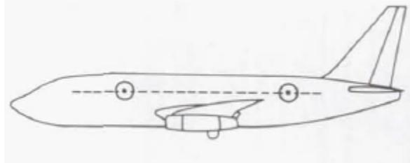
Figure 1. Boeing 737 Forward and Aft Measurement Locations
