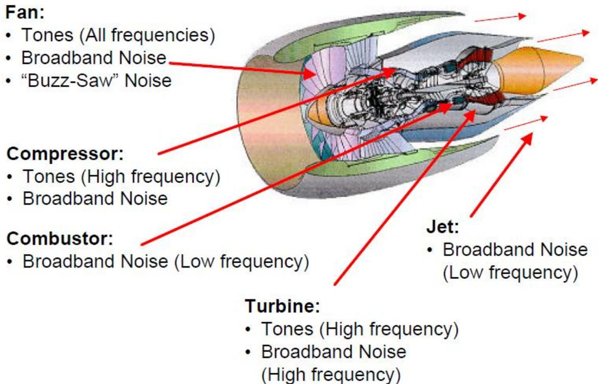
Figure A-1. Turbofan Engine Noise Sources
