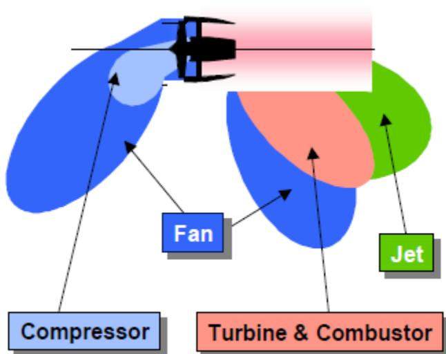
Figure A-2. Turbofan Engine Radiation Pattern
