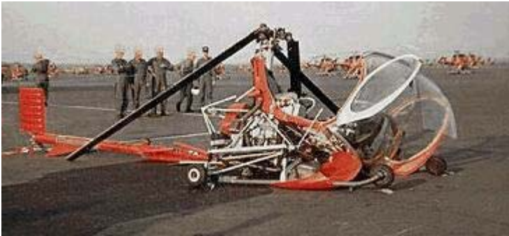
Figure 4. A TH-55 Destroyed by Ground Resonance
