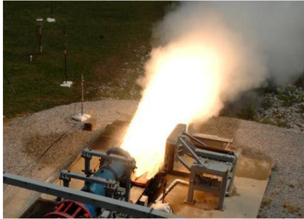
Figure 2. Solid Rocket Motor, Static Fire Test.
