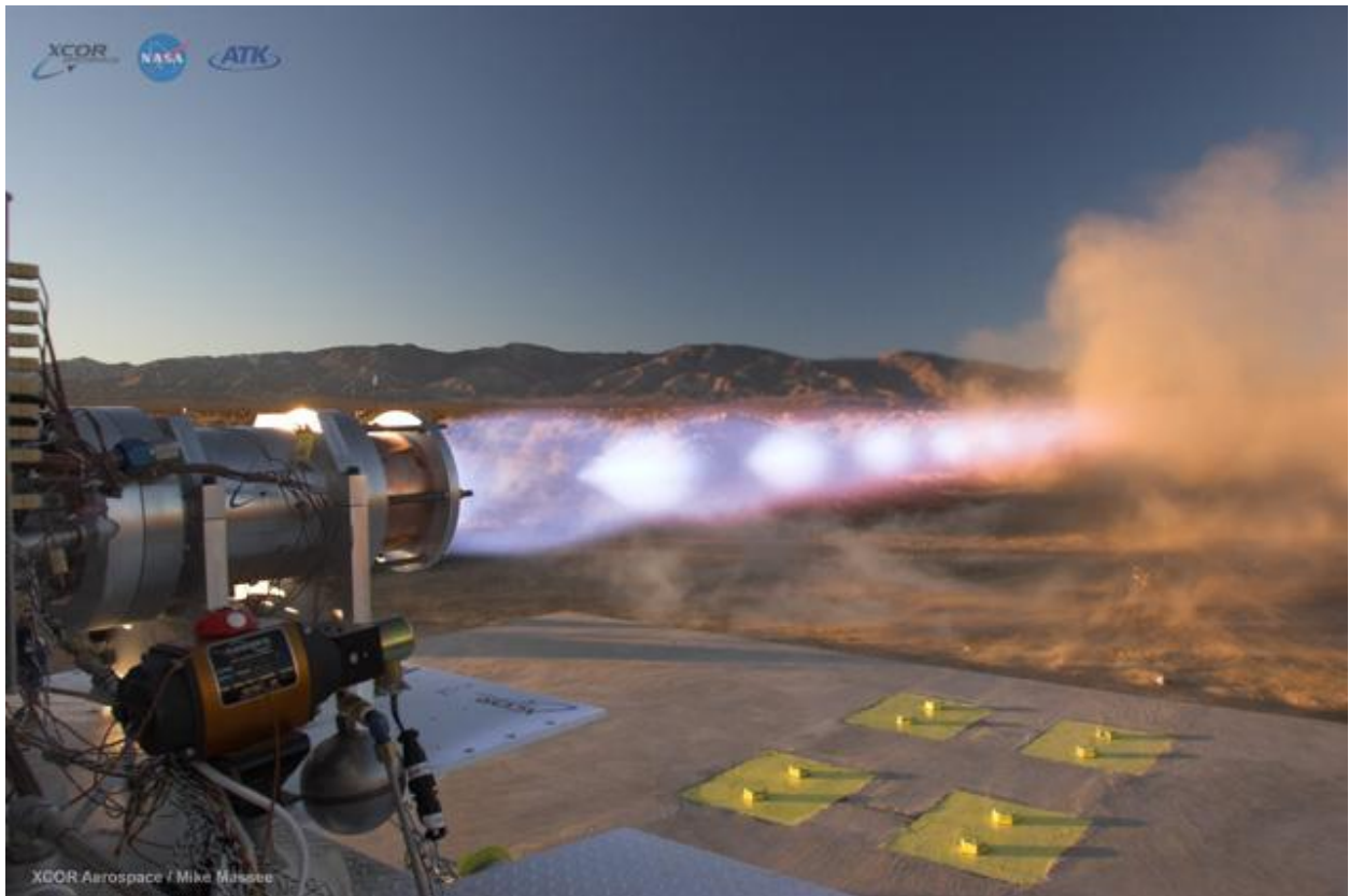
Figure 1. XCOR Aerospace, Liquid Oxygen/Methane Rocket Engine, Test Firing
