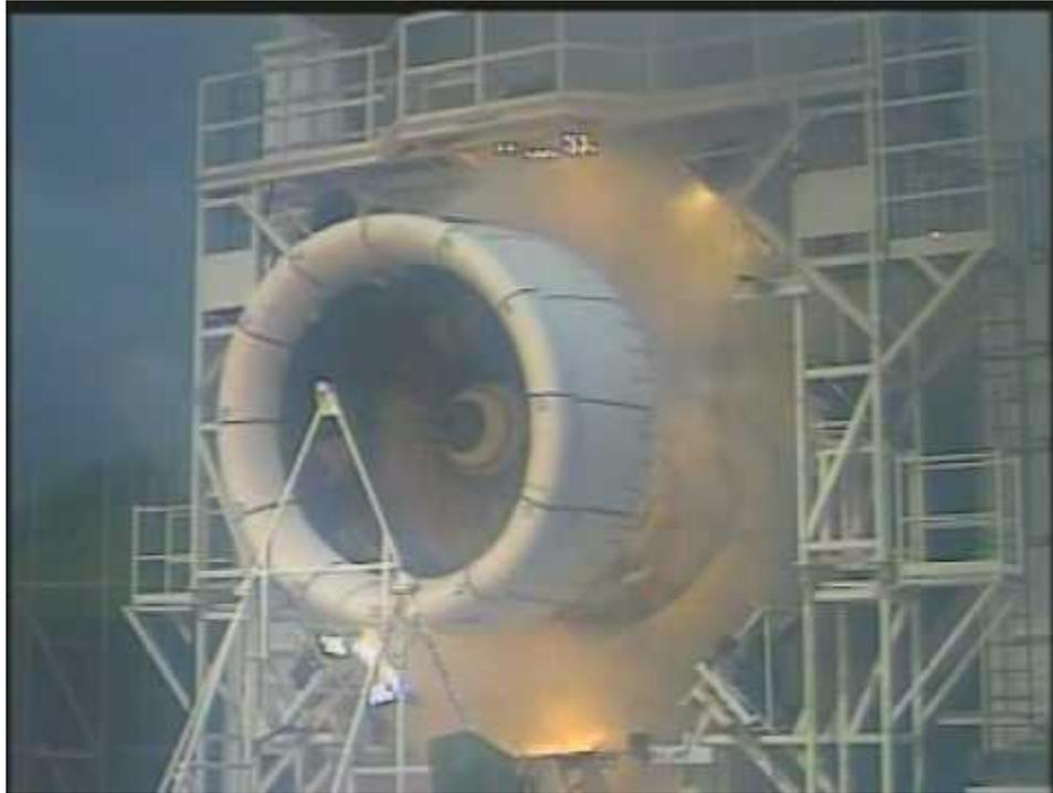
Figure 18.7. Rolls Royce Engine Blade-off Test
