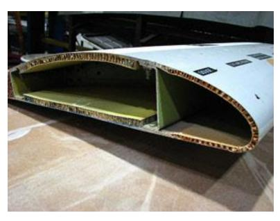
Figure 14.4. Honeycomb Sandwich Structure, Boeing 747 Fore Flap
