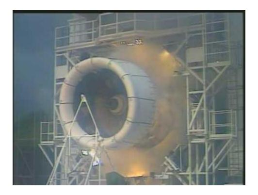
Figure 18.7. Rolls Royce Engine Blade-off Test
