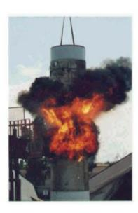
Figure 26.41. Stage Separation Ground Test, Linear Shaped Charge
