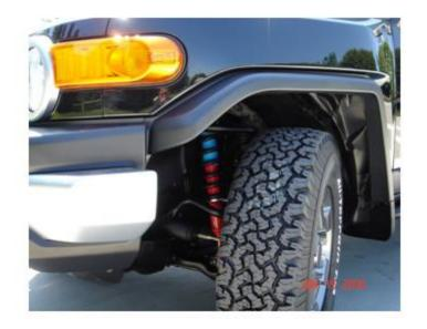
Figure 15.3. Truck Shock Absorber
