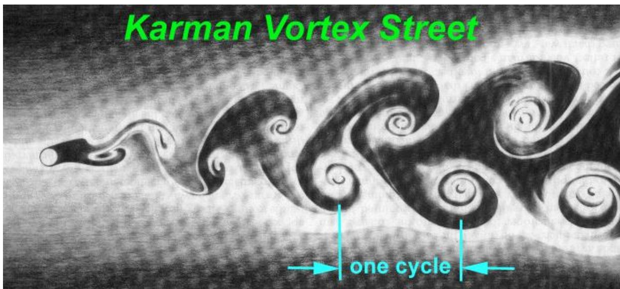
Figure 7.3. Vortex Shedding around a Spherical Body
