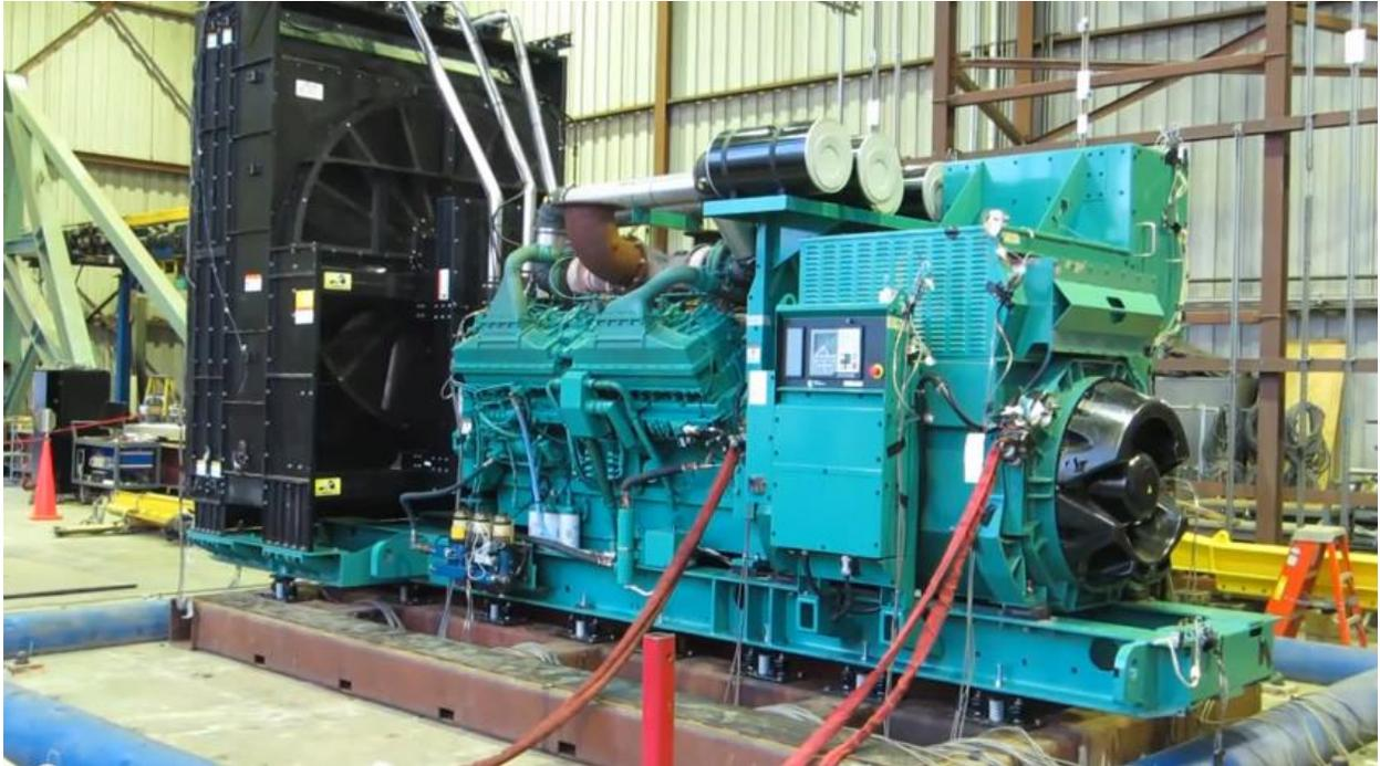
Figure 26.37. Electrical Power Generator Seismic Shock Test
