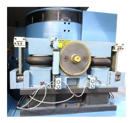
Figure 17.9. Vibration Shaker with Black Air Cushion Mounts
