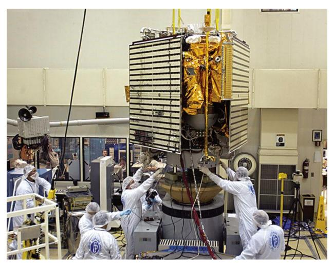
Figure 34.1. Shaker Table Vibration Test
