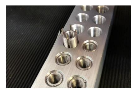
Figure 32.4. Keenserts (useful photo but not a test fixture)
