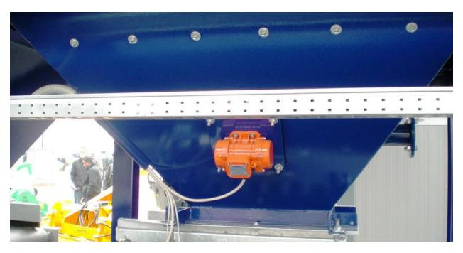
Figure 18.5. Eccentric Mass Vibrator Mounted Externally on Hopper
