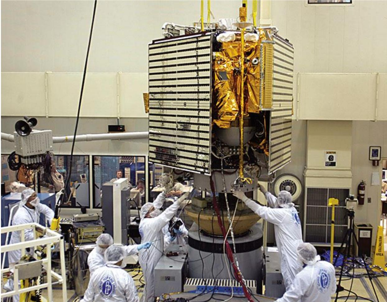
Figure 34.1. Shaker Table Vibration Test
