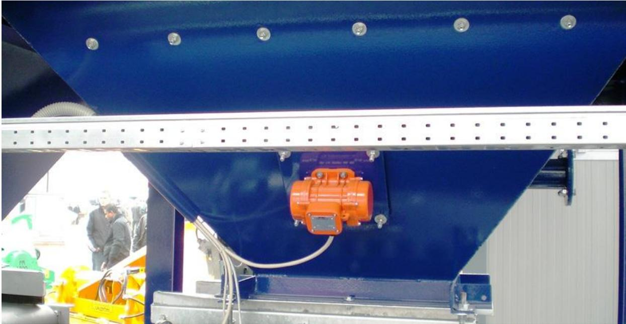
Figure 18.5. Eccentric Mass Vibrator Mounted Externally on Hopper
