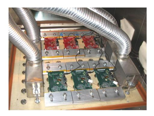
Figure 21.10. HALT/HASS Testing of Circuit Boards, Combined Thermal Cycling and Vibration
