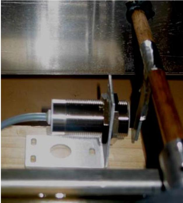
Figure 30.10. Non-contact Relative Displacement Sensor
