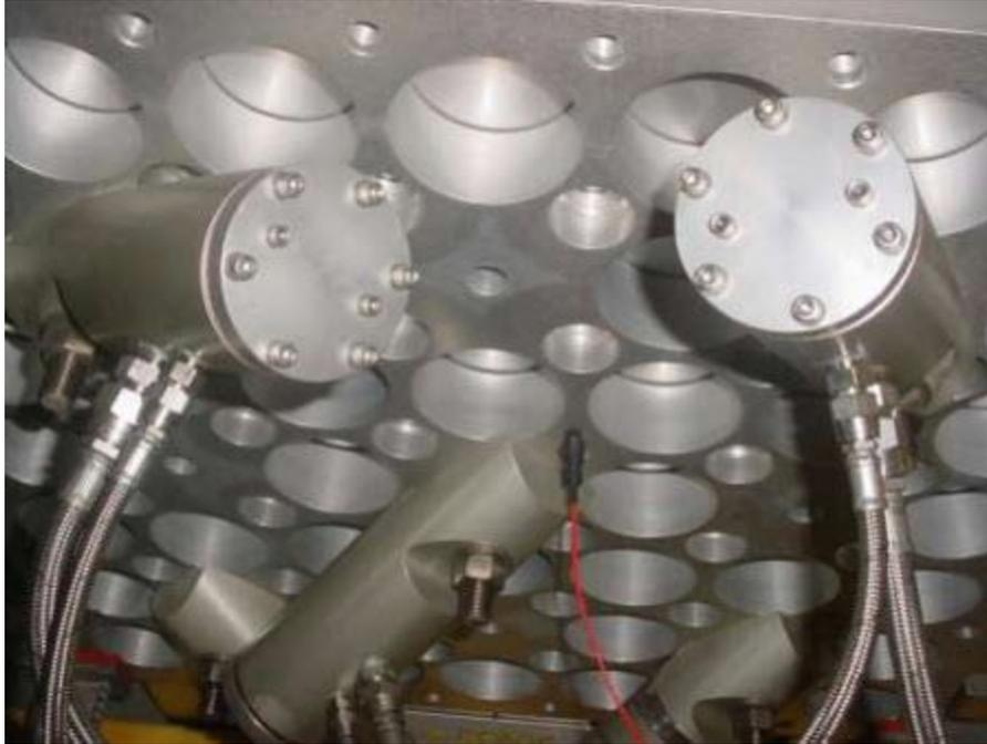
Figure 21.11. HALT/HASS Chamber Vibration Impactors
