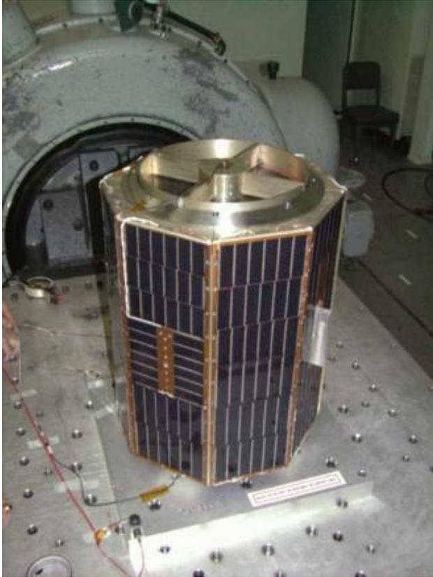
Figure 6.9. Shaker Table Testing, Lateral Base Excitation
