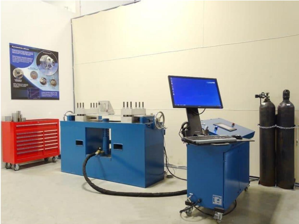
Figure 26.55. Commercial Shock Beam (photo courtesy of MGA)
