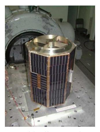
Figure 6.9. Shaker Table Testing, Lateral Base Excitation
