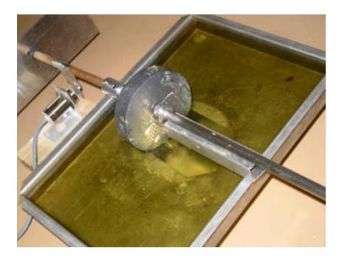
Figure 30.11. Ballast Mass Partially Submerged in Oil
