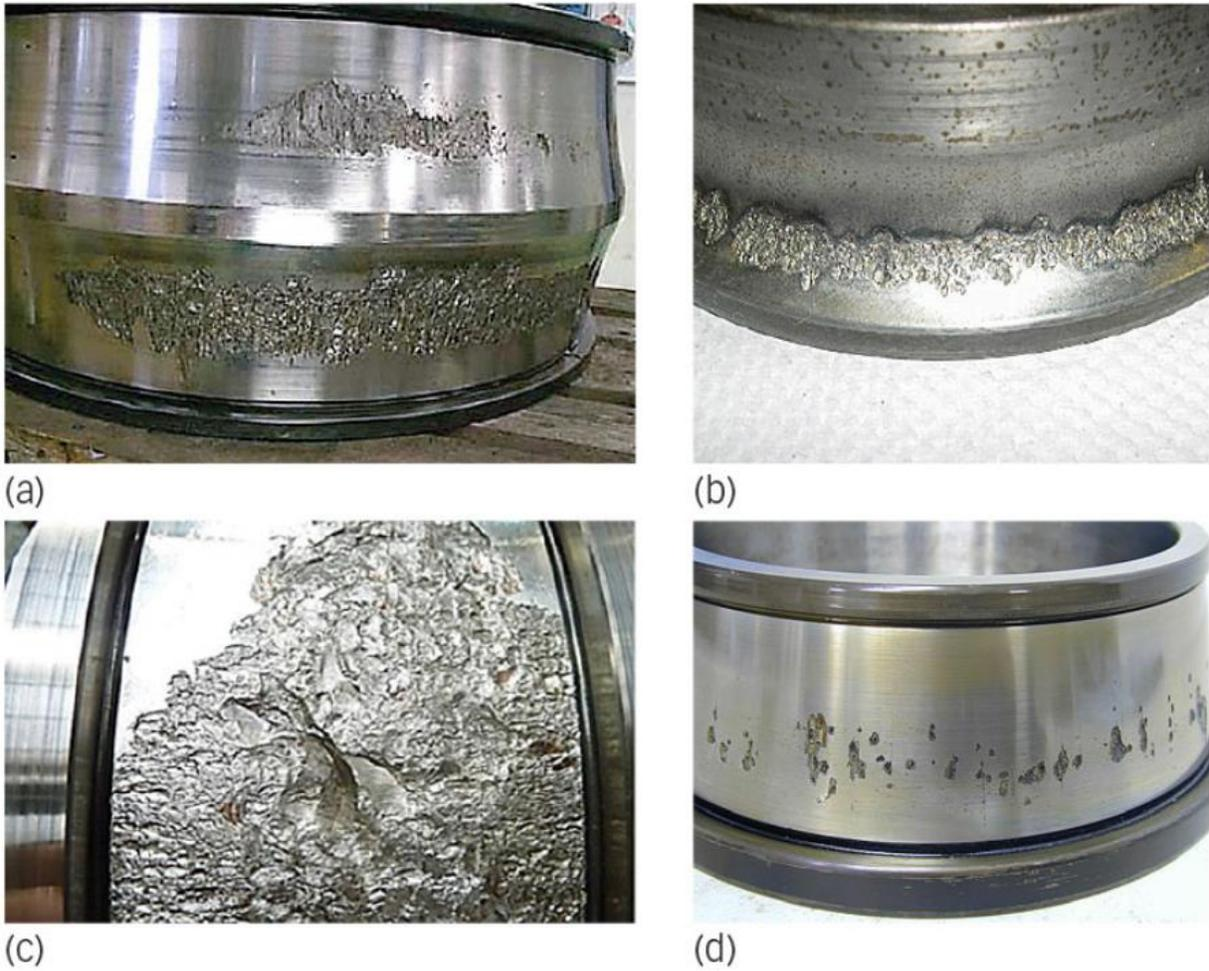
Figure 19.4. Premature Bearing Failures (Image courtesy of Evolution Magazine from SKF)
