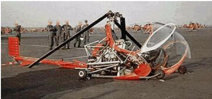
Figure 17.7. TH-55 Osage, Destroyed by Ground Resonance
