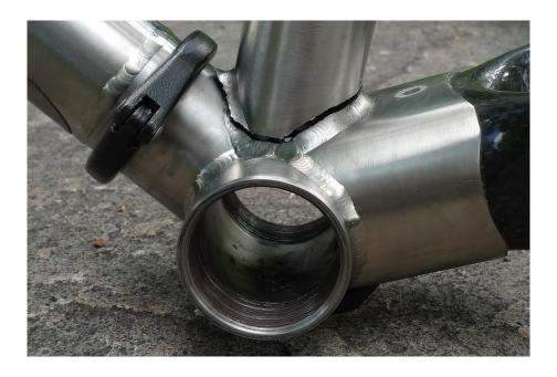
Figure 4.8. Mountain Bike Frame Fatigue Crack in Welded Joint
