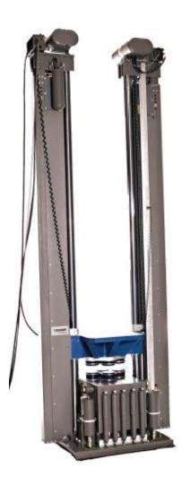
Figure 26.11. Drop Shock Test Machine, Initial Velocity Excitation
