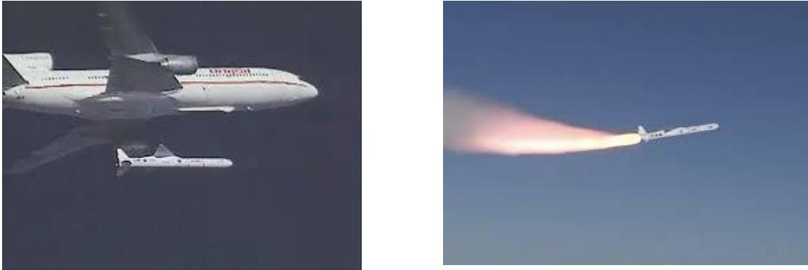
Figure 15.12. Pegasus Launch Vehicle, Drop & Stage 1 Burn
