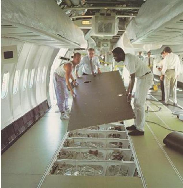
Figure 14.3. Honeycomb Panel, Aircraft Cabin Floor
