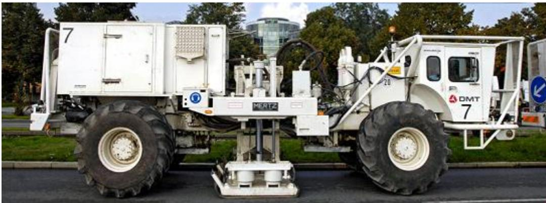
Figure 6.13. Thumper Truck, Applied Force
