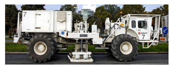
Figure 6.13. Thumper Truck, Applied Force
