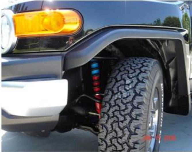
Figure 15.3. Truck Shock Absorber
