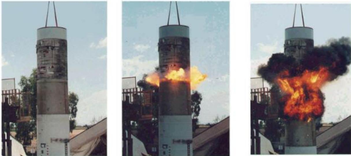
Figure 26.41. Stage Separation Ground Test, Linear Shaped Charge
