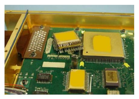
Figure 26.57. Shock Test Case History, Adhesive & Solder Joint Failure
