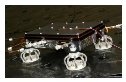
Figure 26.5. Sensor Electronics, Wire Rope Isolators (NASA/JPL photo)
