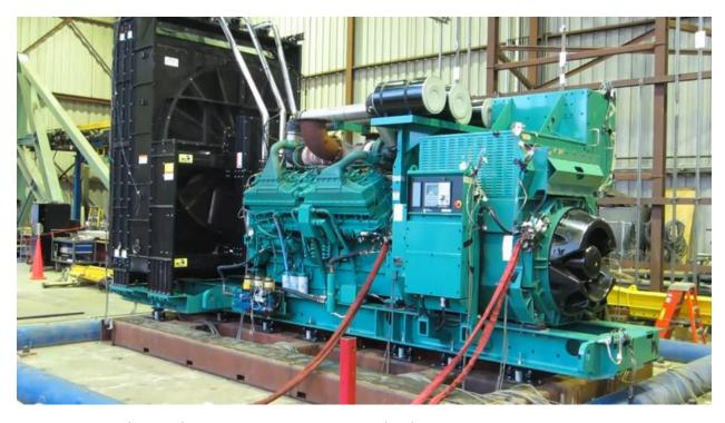
Figure 26.37. Electrical Power Generator Seismic Shock Test
