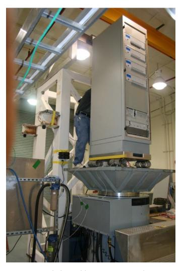
Figure 6.10. Shaker Table Testing, Vertical Base Excitation
