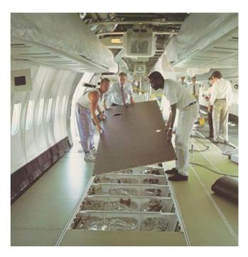
Figure 14.3. Honeycomb Panel, Aircraft Cabin Floor
