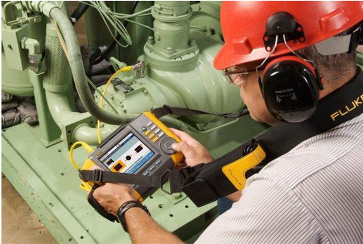
Figure 4.10. Vibration Monitoring for Predictive Maintenance
