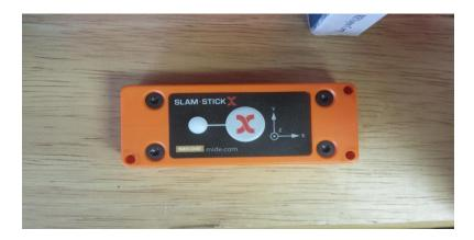
Figure 15.10. Slam Stick X, Triaxial Accelerometer & Data Logger, Shown on Bookshelf
