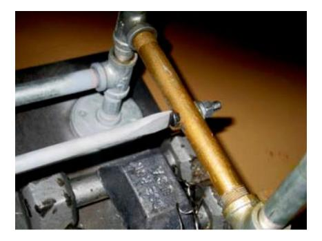
Figure 30.12. Pivot at the End of the Boom
