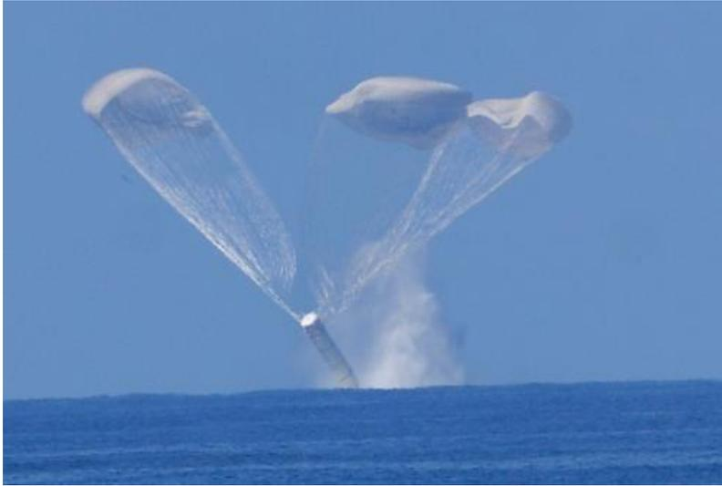
Figure 26.49. Solid Rocket Booster Water Impact Shock
