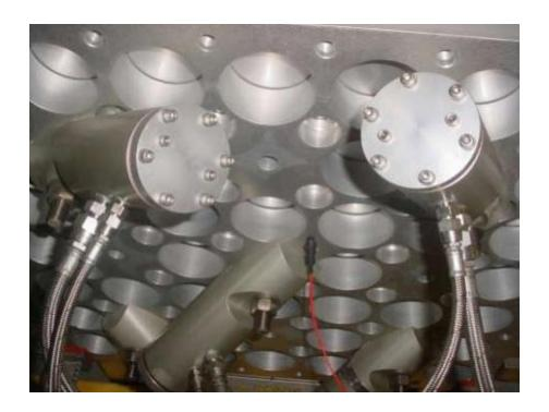
Figure 21.11. HALT/HASS Chamber Vibration Impactors
