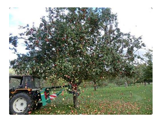
Figure 18.3. Commercial, Tractor-Mounted Tree Trunk Shaker, Apple Harvesting
