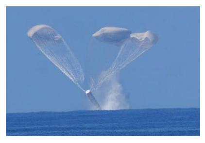
Figure 26.49. Solid Rocket Booster Water Impact Shock
