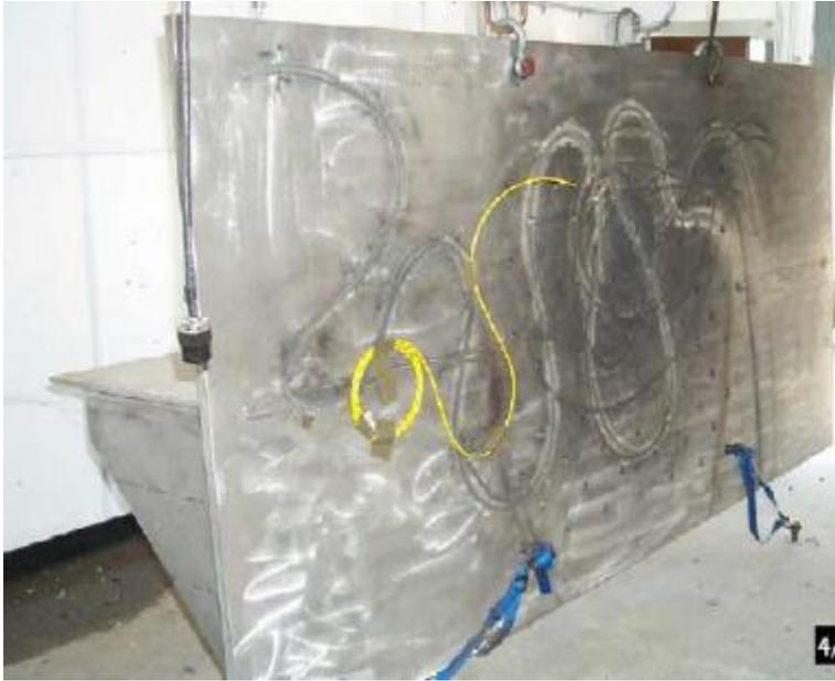
Figure 26.53. Near-Field Shock Simulation using a Plate
