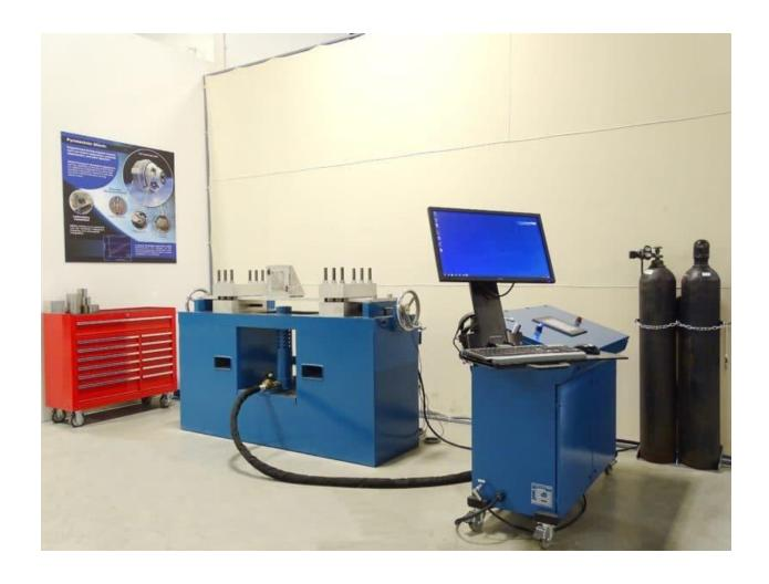
Figure 26.55. Commercial Shock Beam (photo courtesy of MGA)
