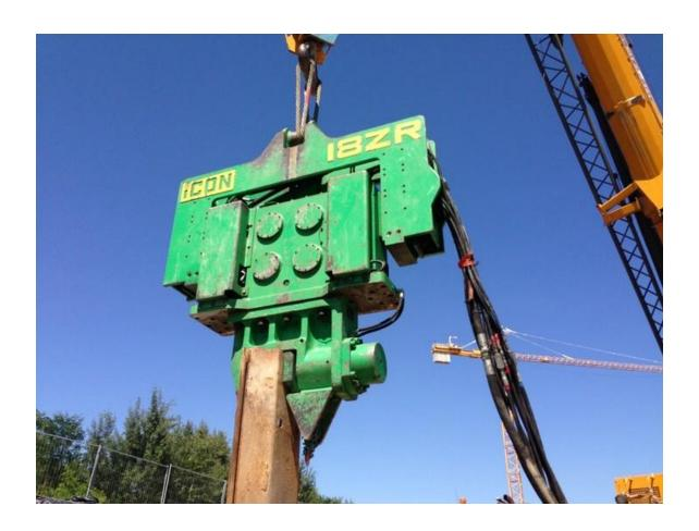
Figure 18.4. Vibratory Hammer Suspended from Crane Boom for Pile Driving
