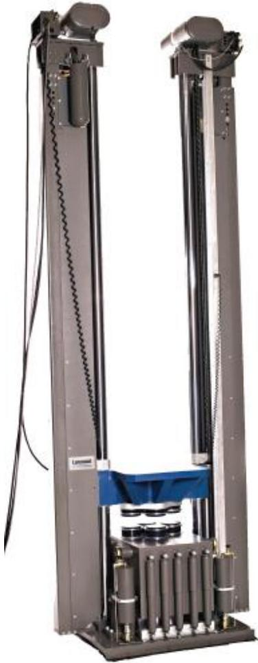
Figure 26.11. Drop Shock Test Machine, Initial Velocity Excitation
