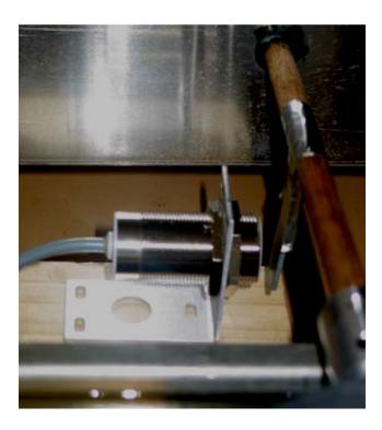
Figure 30.10. Non-contact Relative Displacement Sensor
