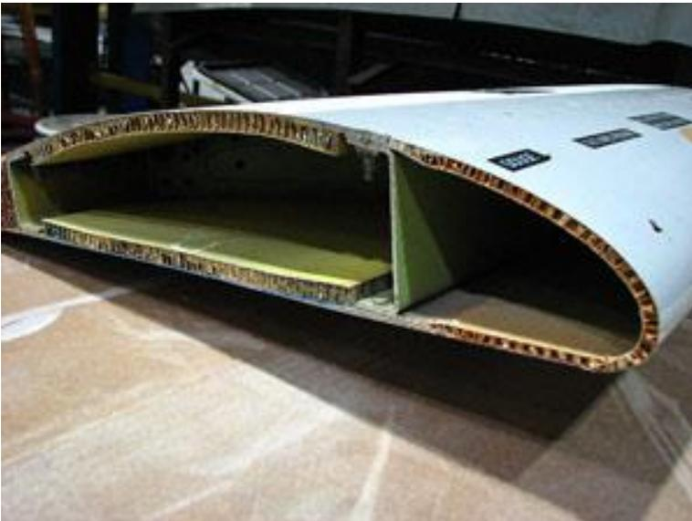
Figure 14.4. Honeycomb Sandwich Structure, Boeing 747 Fore Flap
