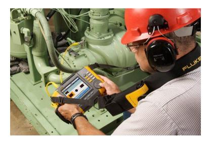
Figure 4.10. Vibration Monitoring for Predictive Maintenance
