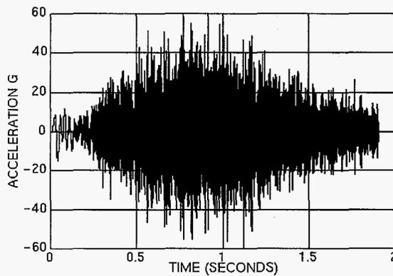
Figure 5: Acceleration History for Transient Random Test Specification
