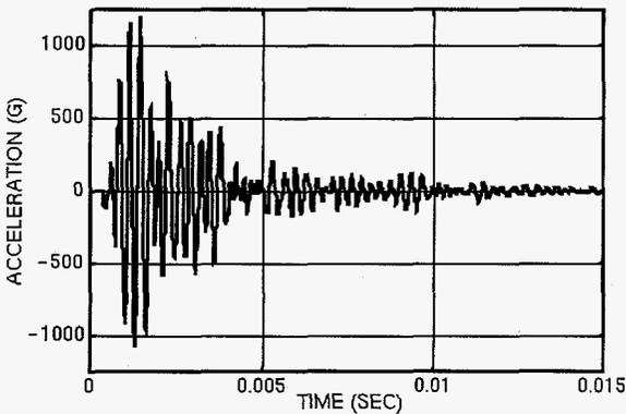
Figure 6: Acceleration History for Severe Field Environment
