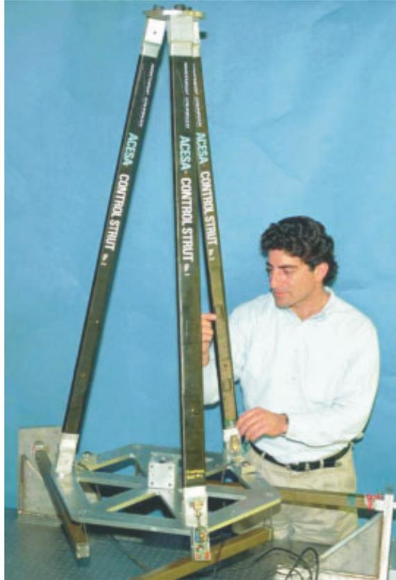
**Figure 14. Smart Structures Experimental Test Set active beam isolator**
