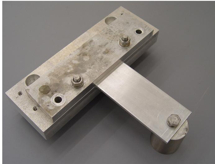
Figure 6.12. Cantilever aluminum plate
