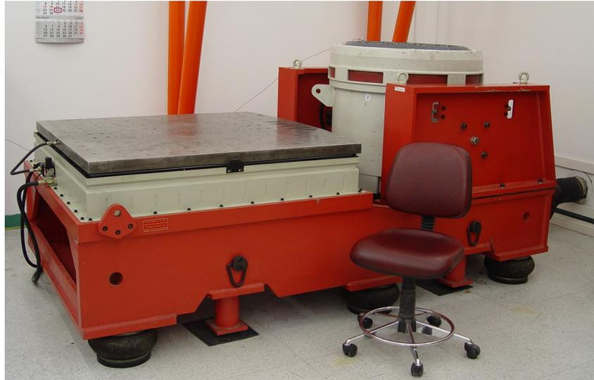
Figure 6.1. Vibration test system
