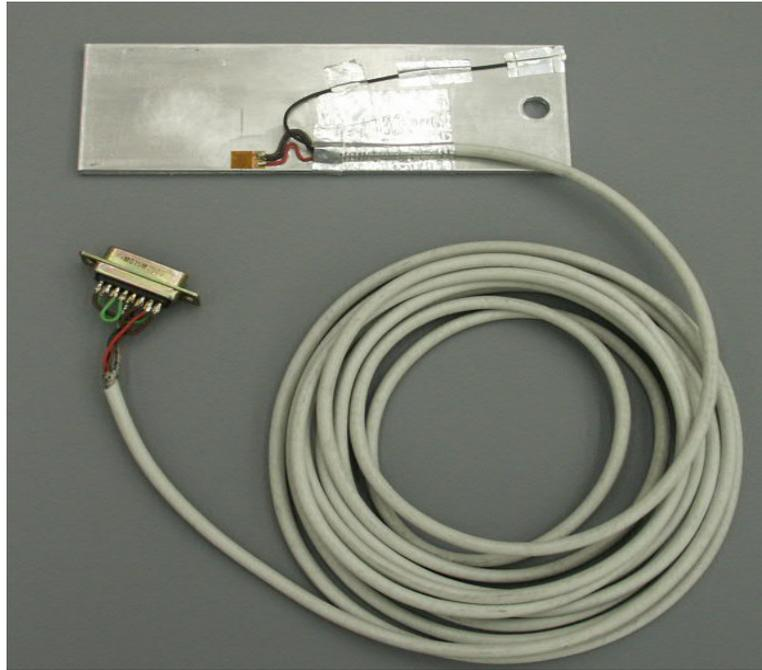
Figure 6.17. Aluminum test specimen, cable and the connector
