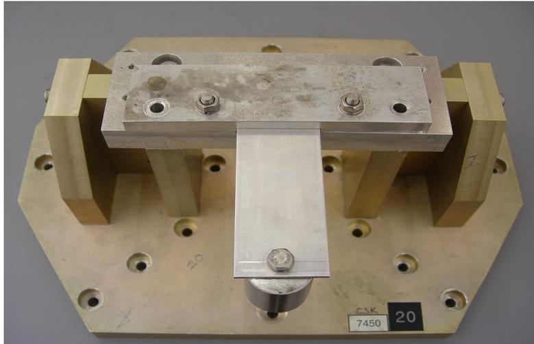
Figure A.12. The notch placed on the bottom surface of the aluminum plate
