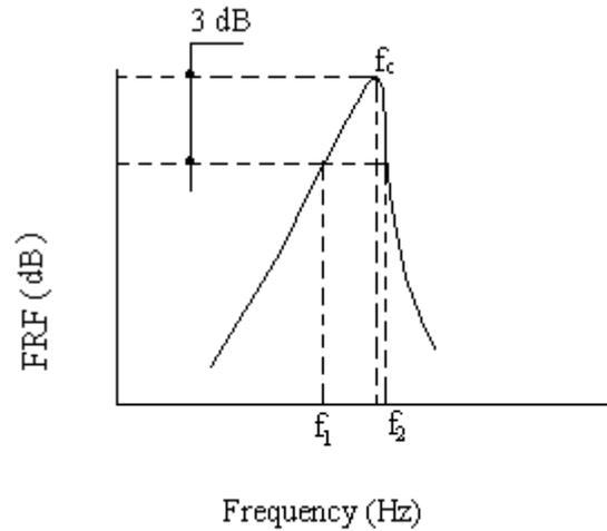
Figure 1. Typical frequency response function of Oberst bar
