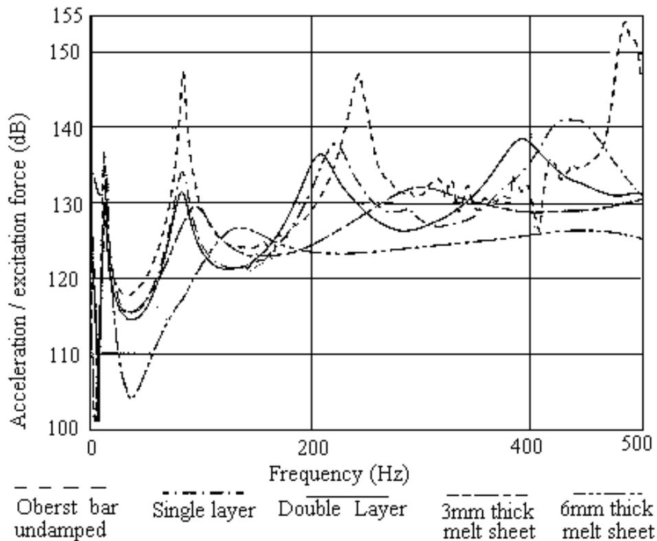
Figure 3. Frequency response function of different configuration of Oberst bar
