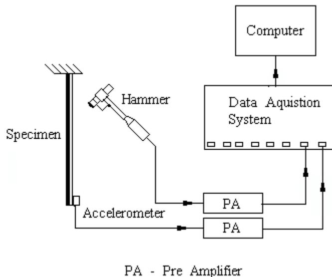
Figure 2. Experimental set-up for damping loss factor measurement.
