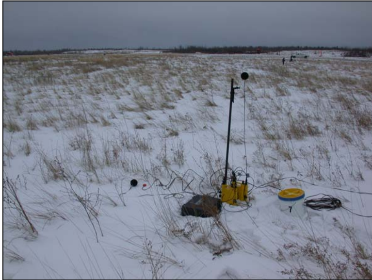
Figure 20. Photo of Test 6 experiment, measurements for propagation with a sintered snow cover present (Fort Drum, NY, 2004). Two high pressure microphones are visible with their black round foam wind screens. Two orange geophones were also installed at the surface of the snow cover itself. The yellow boxes are waterproof digitizers, and the black case and white bucket are used to protect the power supplies from the weather. Although there are many bushes poking through the snow, the snow cover at this site was continuous and relatively deep (ranging from 8 to 25 cm) compared to the Test 5.
