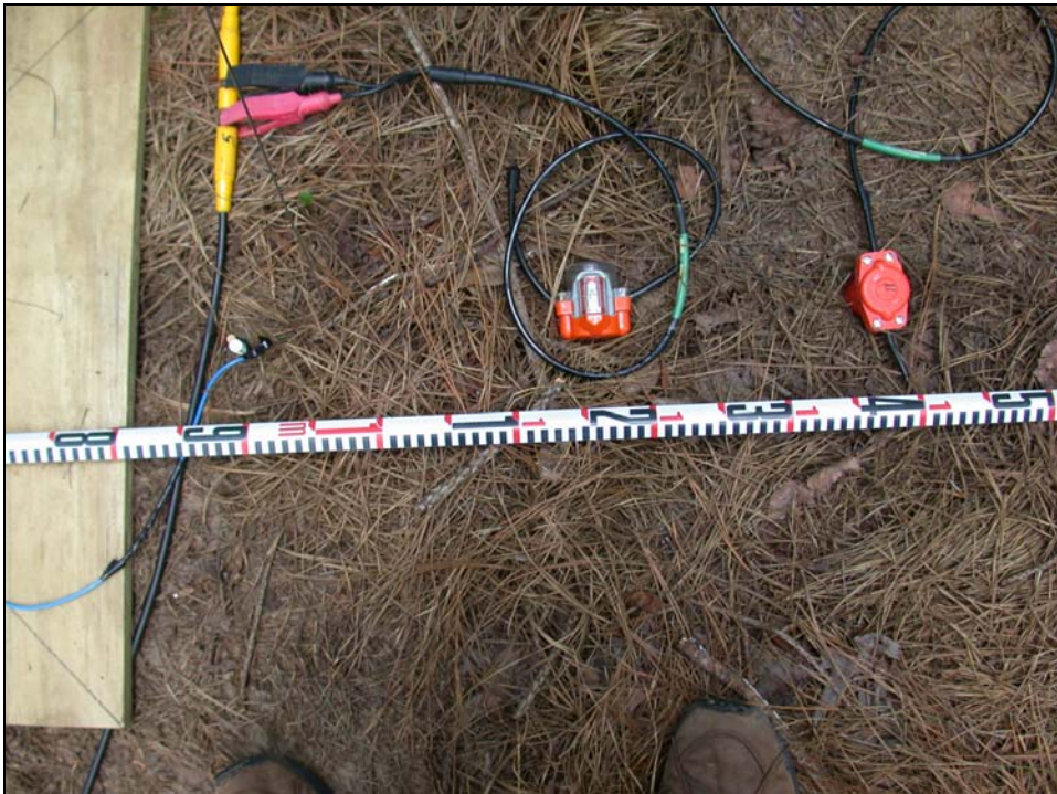
b. Close view of typical ground conditions within the forest, showing a horizontal and a vertical component geophone installed in the ground. The tick marks on the scale are in cm, the large divisions and numbers indicate 10-cm intervals.
