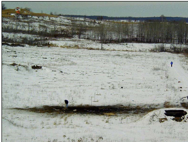
b. Test 5 experiment after some shots were detonated. The large dark patch with a person standing within is the location where the C4 charges were detonated. The sensor array extends in a straight line away from the camera, starting near that point. The ground was very rough in this location, and the snow cover was not continuous or uniform.
