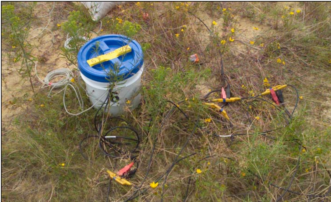
c. Two orange geophones installed at the 100-m sensor location, one sensitive to vertical ground motion and the other sensitive to horizontal motion. These sensors are the same distance away from the source as the pressure sensors shown in 7b.
