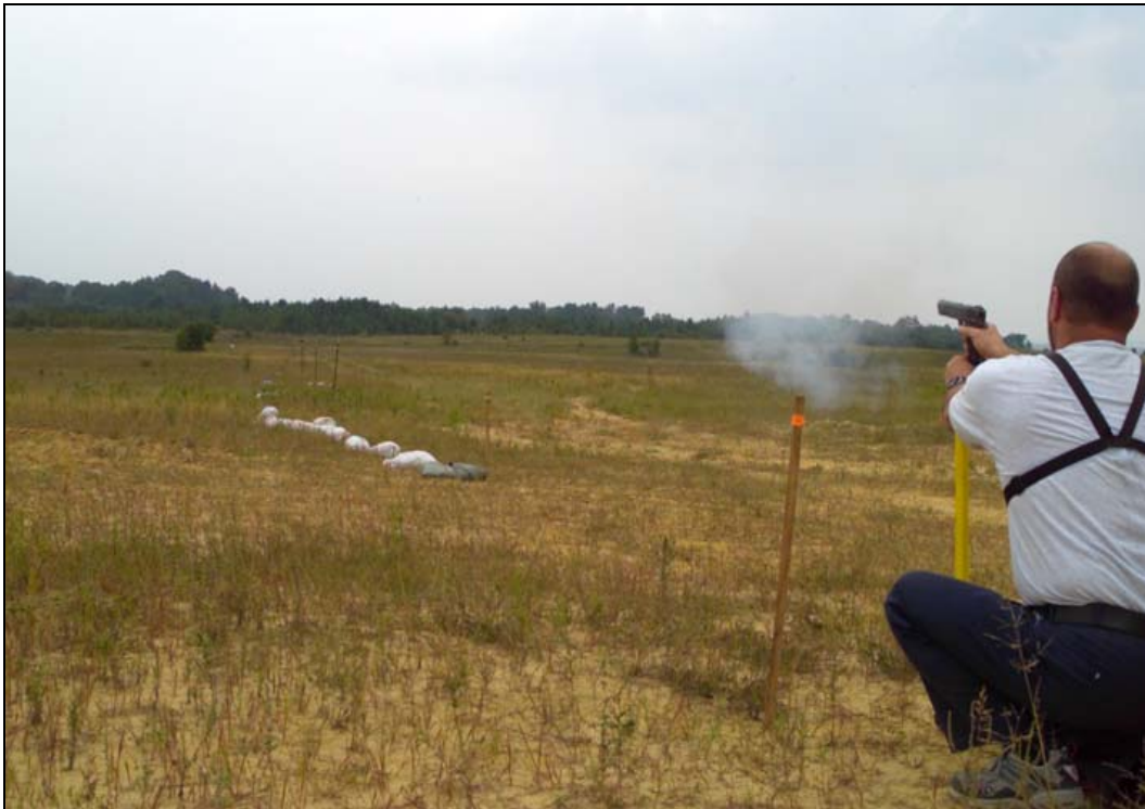
a. Blank pistol shot being fired at the C4 source location. Sensors in a linear array are spaced 10–240 m from the source point. The white sand bags were used to protect some of the sensor cables, as a maximum charge size of 73 kg might have damaged them. This photo is intended to show the general ground and vegetative conditions during the tests. The sensors used in this report were 100 m or more from the source location, starting at about same distance away as the small tree visible to the left of the photograph.
