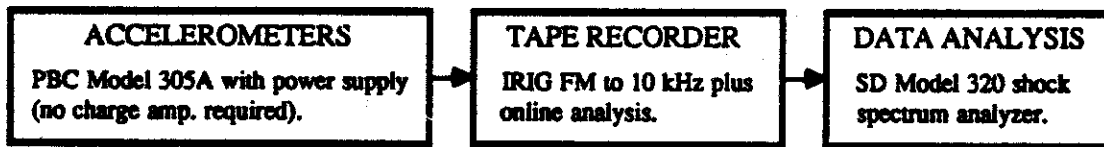
FIGURE 9. Data Acquisition And Analysis System For NTS RMUC Tests.
