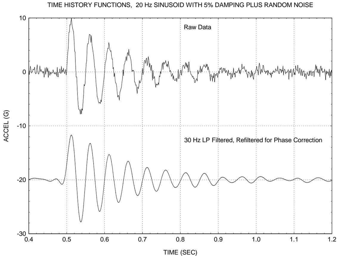
Figure 3. Transient Example with Refiltering
