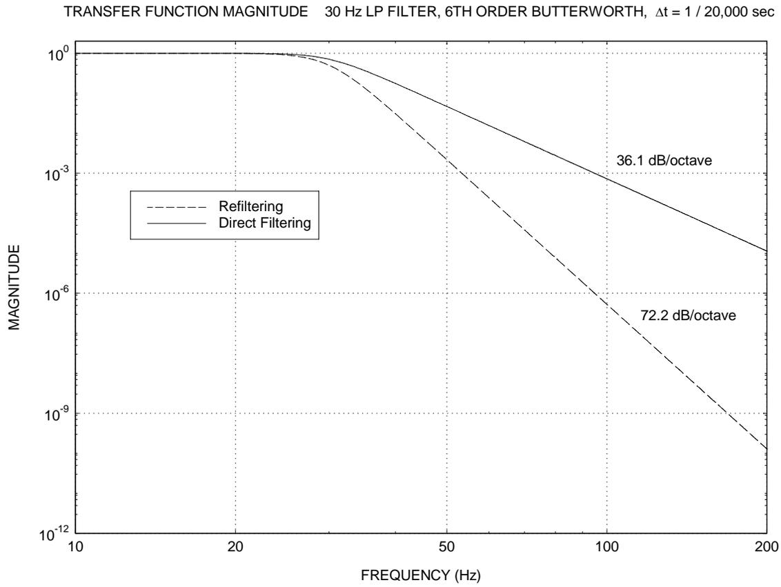
Figure 6. Roll-off Slopes
