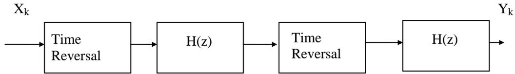
Figure 1. Refiltering Diagram
