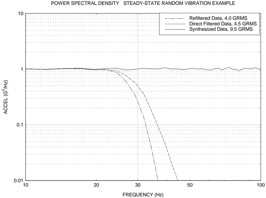
Figure 4. Steady-State Example
