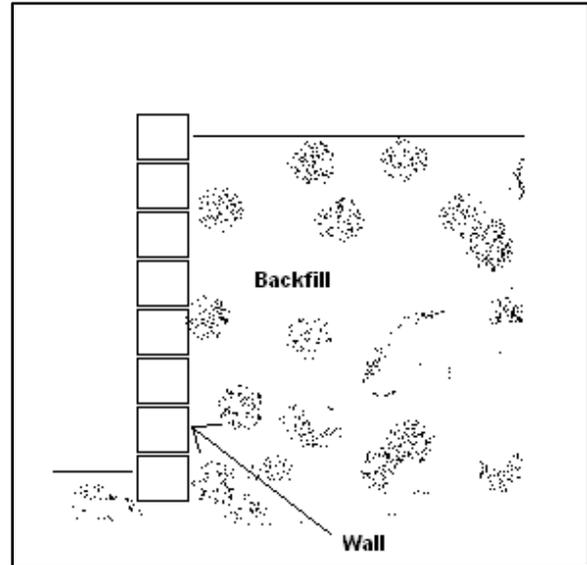
**Figure 8:** Block and mortar wall (no reinforcements).
