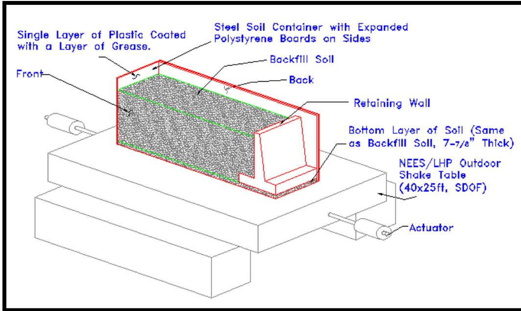
**Figure 3:** Shake table setup for the retaining wall specimen without a sound wall barrier.
