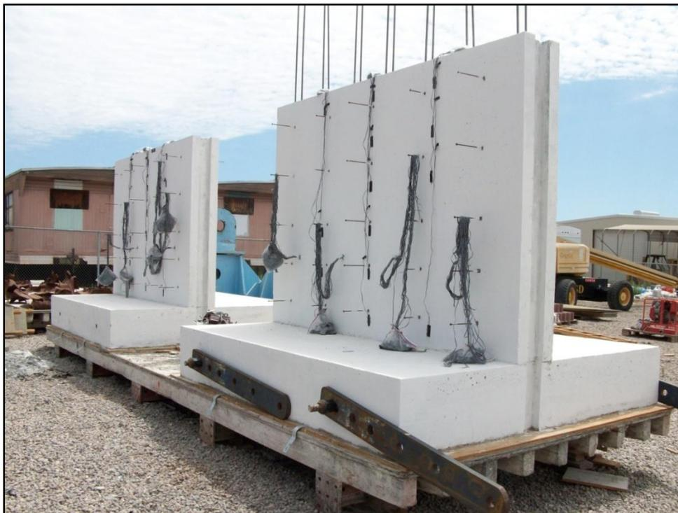
**Figure 4:** Photo of the retaining walls with strain gauges attached. Note the rebars for the infill sound barrier on top of the nearest wall.
