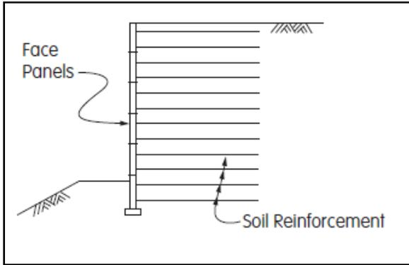
**Figure 6:** Mechanically Stabilized Earth (MSE) wall with panels. These types of retaining structures are designed for large wall heights and are capable of very high performances (Reinforced Earth Company®).
