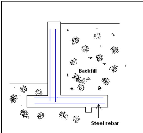
**Figure 7:** Reinforced concrete gravity-cantilever wall.
