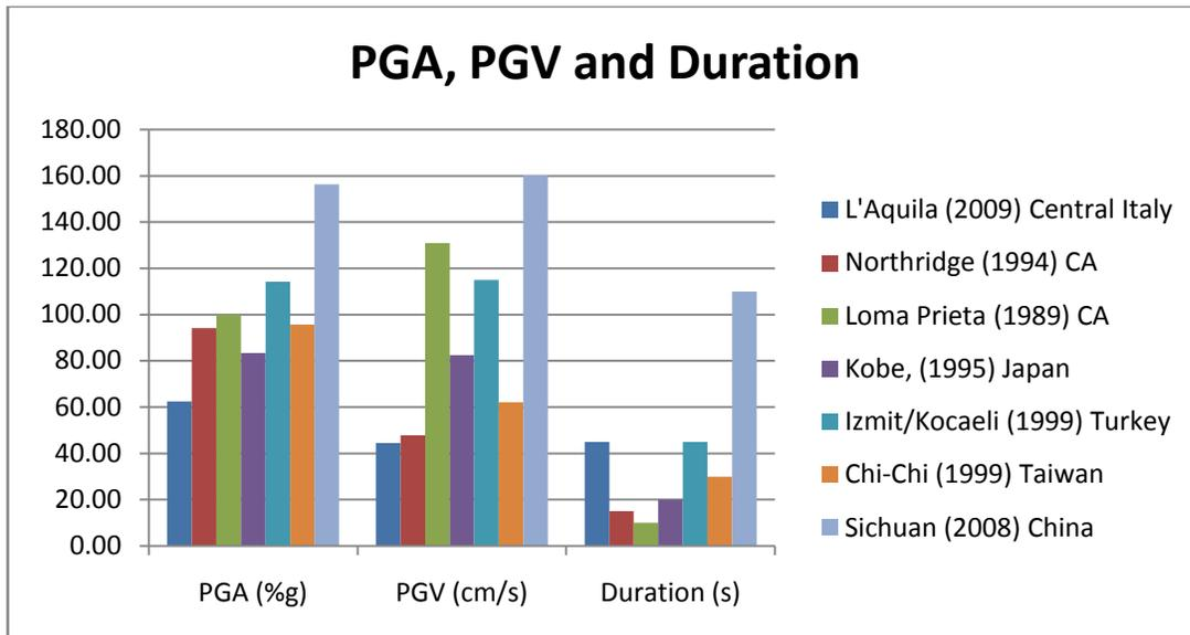
**Figure 5:** Side by side comparison of the peak ground acceleration (PGA), peak ground velocity (PGV) and the *duration* of each earthquake.
