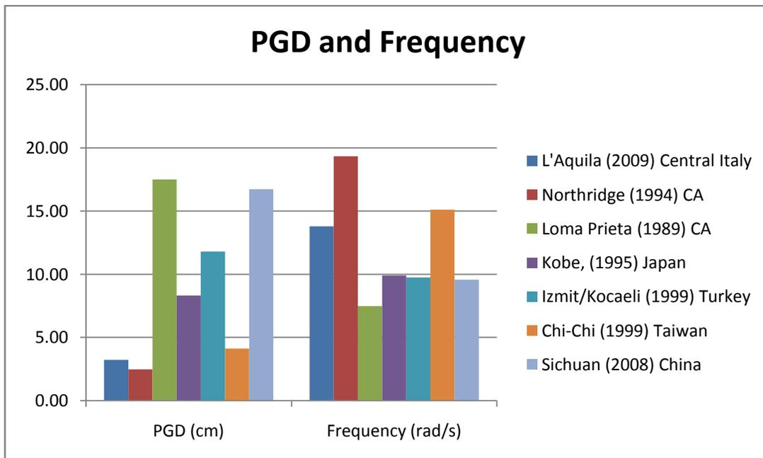
**Figure 4:** Side by side comparison of the peak ground displacement (PGD) and the frequencies of the earthquakes.
