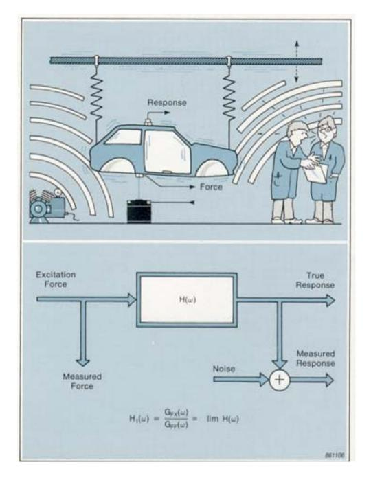
An important point about  $H_1$  is that random noise in the output is removed during the averaging process of the Cross Spectrum. As the number of averages is increased,  $H_1$  converges to the true H.
