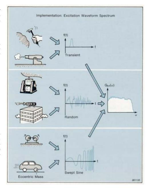
**Spectrum control** is the capacity to limit the excitation to the frequency range of interest.
