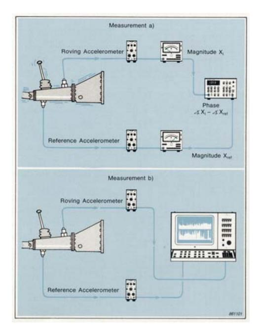
The operational deflection shape represents the absolute deflection of a structure due to the unknown but real forces. The deflection shape does not give any information about the independent dynamic properties of the system. Information cannot therefore be obtained about deflections due to other forces, or at other frequencies.
