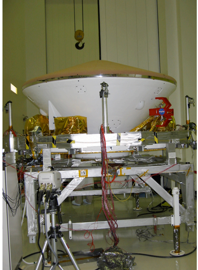
Figure 3. MER Spacecraft Configuration for V-band Separation Test
