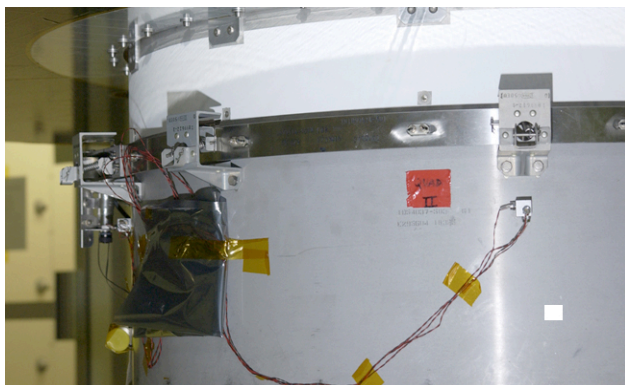
Figure 4. Shock Response Accelerometer Locations for MER#2 V-Band Separation Test (Response Accelerometers Mounted above V-Band in MER#1 Launch Separation Test)
