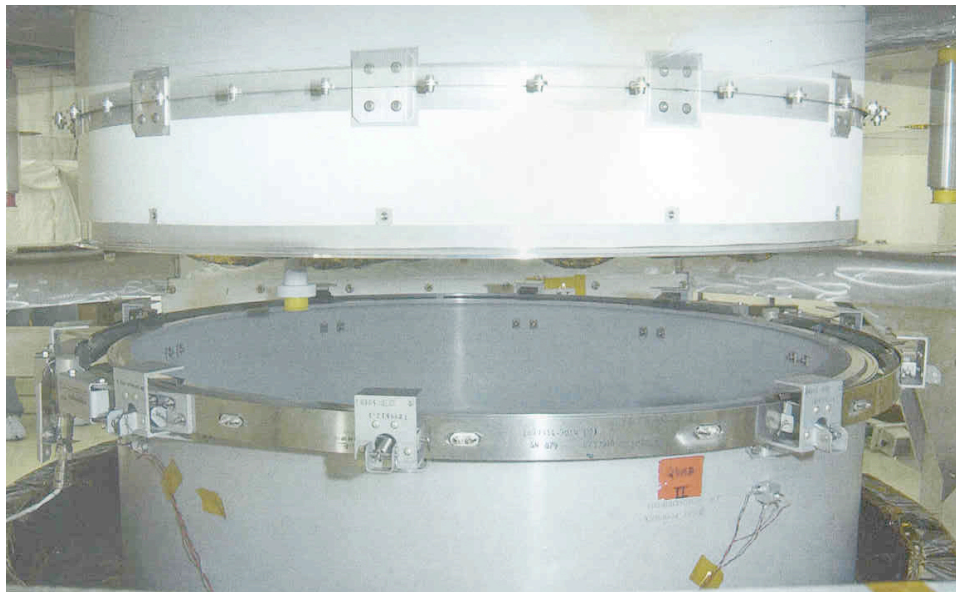
Figure 1. MER V-Band Assembly after Separation
