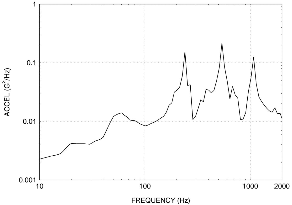
Figure 1. Flight Power Spectral Density
