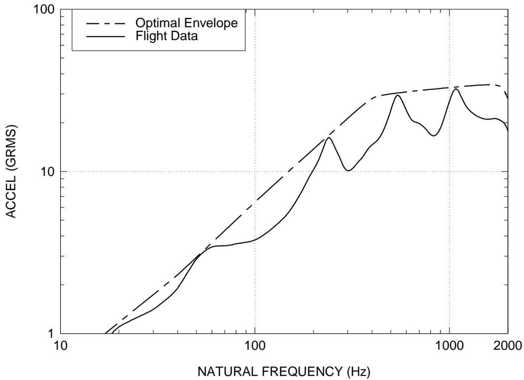
Figure 5. Optimal Envelope Vibration Response Spectrum
