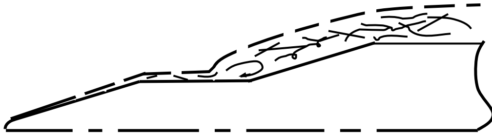
Figure 4. Cone-Cylinder Geometry with Separated Flow near Compression Corner, Subsonic
