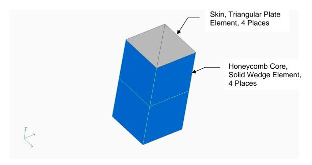
Figure D-2. Manually Constructed Laminate for FEA
