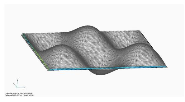
Figure D-4. Typical FEA Mode Shape, fn = 362 Hz
