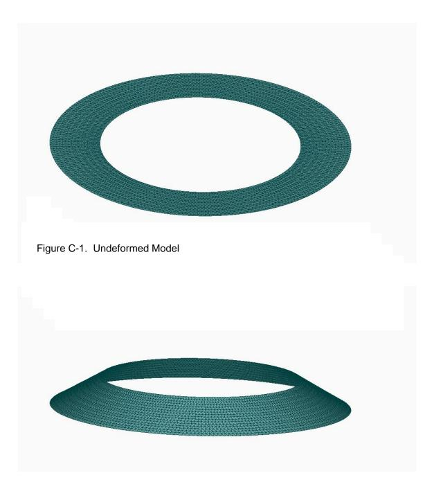
Figure C-2. Mode 1, fn = 39.6 Hz
