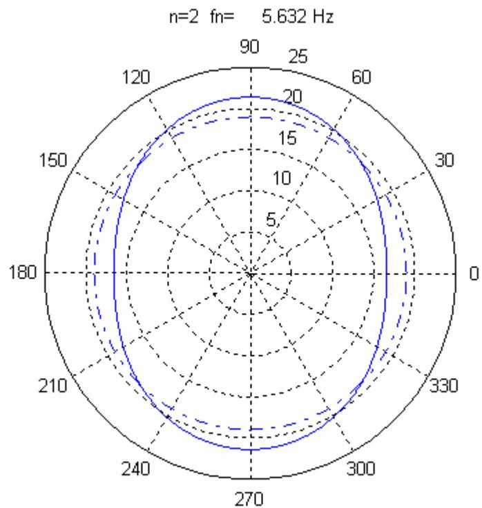
Figure A-2.  $n=2$ , Freq = 5.63 Hz, Flexural Mode
