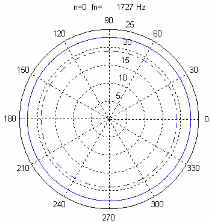
Figure A-7.  $n=0$ , Freq = 1727 Hz, Extension Mode
