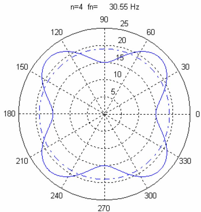
Figure A-4.  $n=4$ , Freq = 30.6 Hz, Flexural Mode
