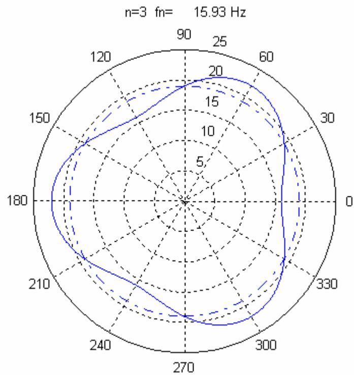
Figure A-3.  $n=3$ , Freq = 15.9 Hz, Flexural Mode
