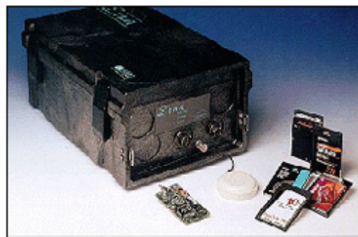
Figure 5.13. Example of a recorder make specifically for strong motion, the Kinematics Etna. The round white box in front of the recorder is the GPS antenna and the PCMCIA cards are seen to the right.
