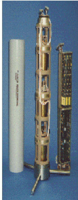
Figure 2.31 A BB borehole sensor model KS-54000 from Geotech instruments. The height is 2.5 m
