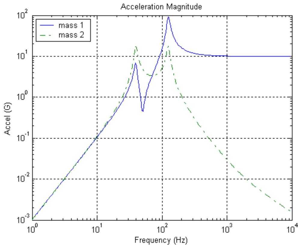
Figure 2. Case with Payload Values:  $m_2 = 200$  lbm,  $k_2 = 5.11 \times 10^4$  lbf/in, (payload  $f_n = 50$  Hz)
