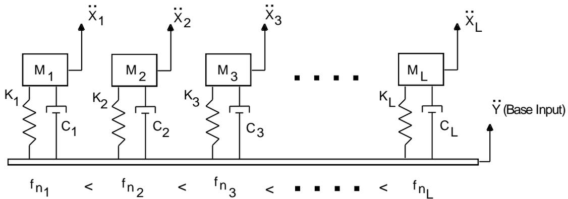
Figure 1. Response Spectrum Model
