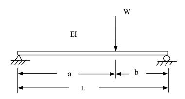
The stiffness at the load point is  $k = \left\{ \frac{3EIL}{a^2b^2} \right\}$ .
